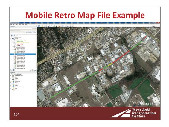
The newer mobile retroreflectometers directly output Google Earth files; these are .kml or .kmz files. These files can be viewed directly in the free Google Earth software.
