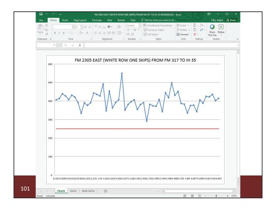
This slide shows a chart associated with a summary data file. The spreadsheet has a chart tab, a data tab (summary data), and a raw data tab. The chart has a horizontal line drawn at 250 indicating the required retro level. All the data are clearly passing on this white skip line.
