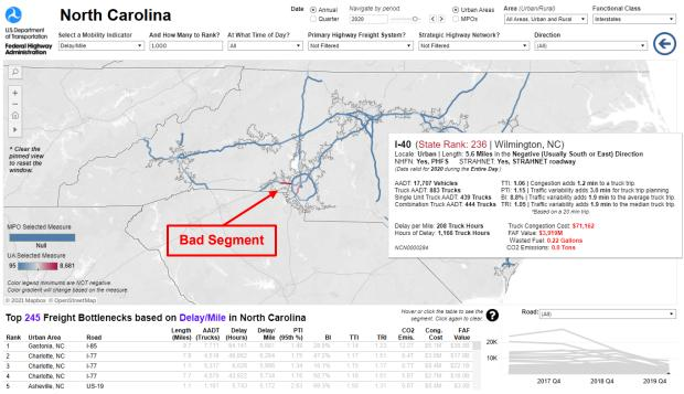
Figure 18: Freight Mobility Bottlenecks Displayed in a Map and Table Using Tableau
