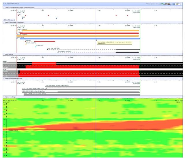
Figure 13: Heat Map and Multilayered Visualization Displaying Incident Congestion Severity
