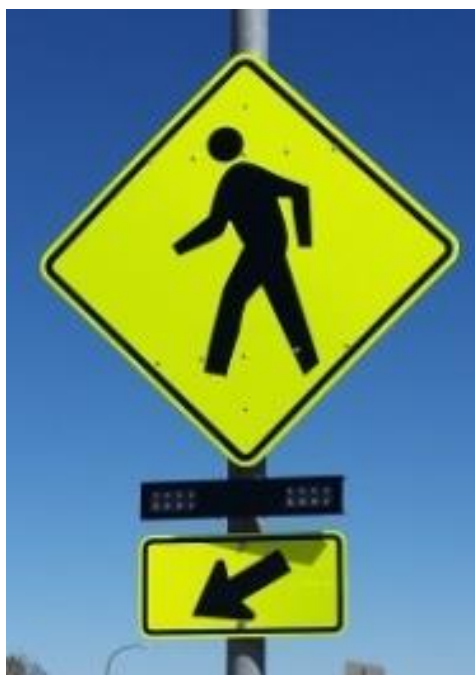
Figure 2. Photo. Example of beacon placed below sign.
