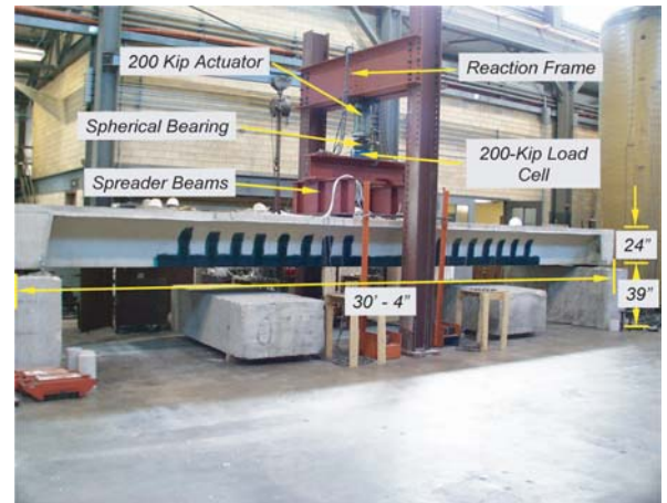
Full-scale testing of FRP-strengthened pan girder bridge.
