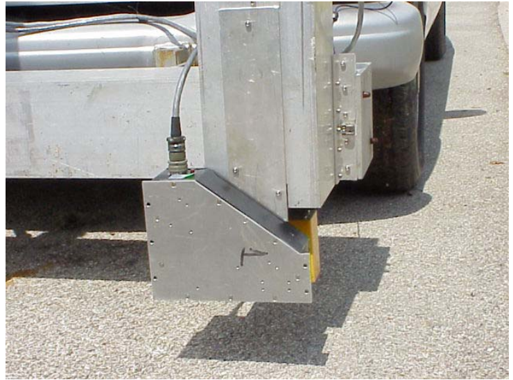
The Laser Texture Measuring System mounted on the front of a multi-purpose pavement testing vehicle
