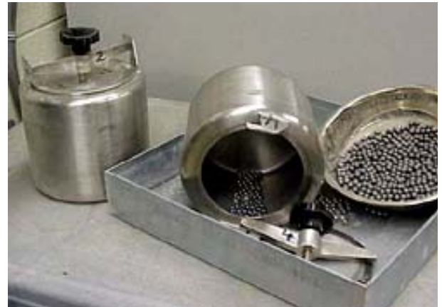
Container and steel balls used in Micro-Deval test
