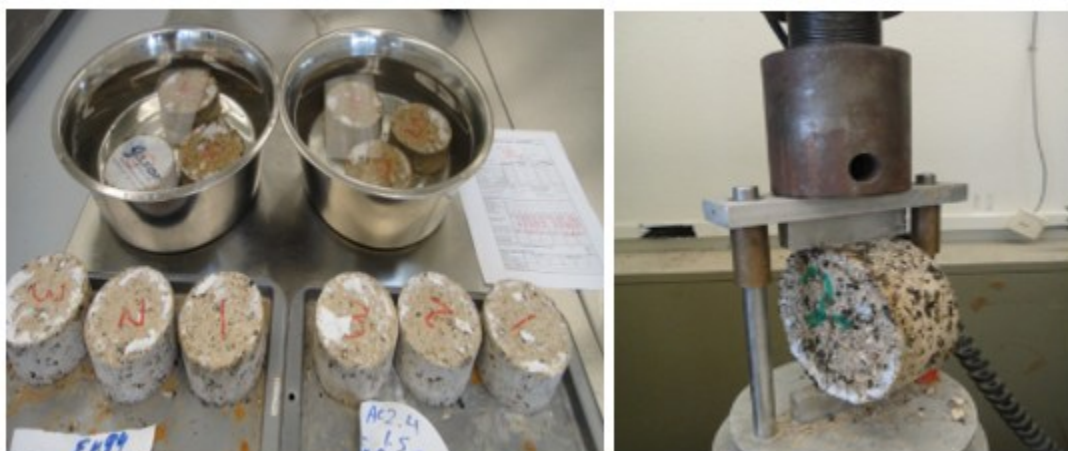
Figure 18. Samples Taken during the Moisture Conditioning and the IDT Test.
