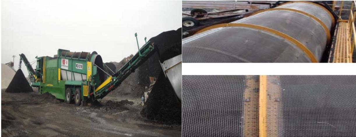
**Figure 6. Screening RAS Using Trommel Screen Machine.**
