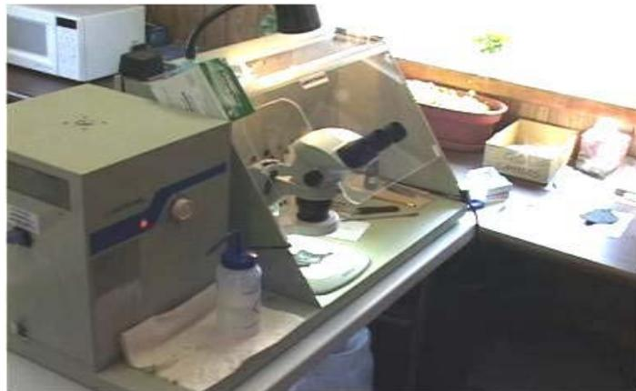
**Figure 3. Setup for Asbestos Testing (after Krivit, 2007).**
