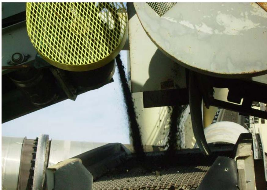
**Figure 15. Vibratory Scalping Screen (after Morton, 2011).**
