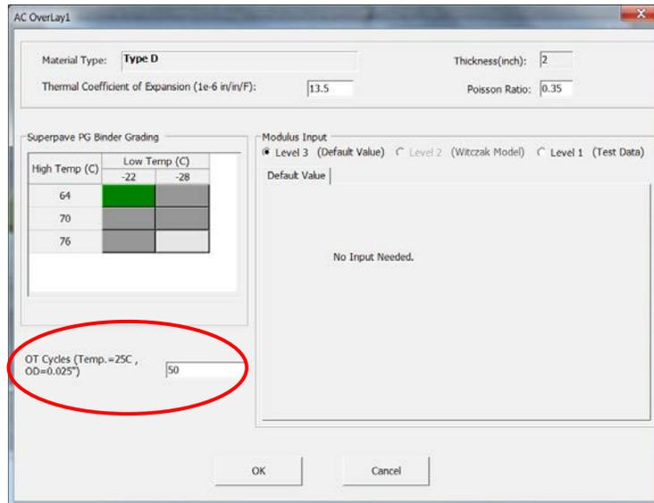
**Figure 9. OT Cycles Input Interface for S-TxACOL.**
