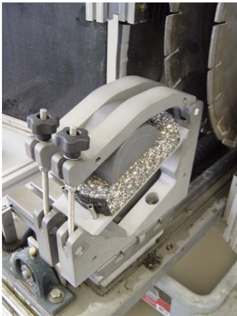
Figure 7. Finished 3 in (76 mm) Wide Specimen after Cutting.
