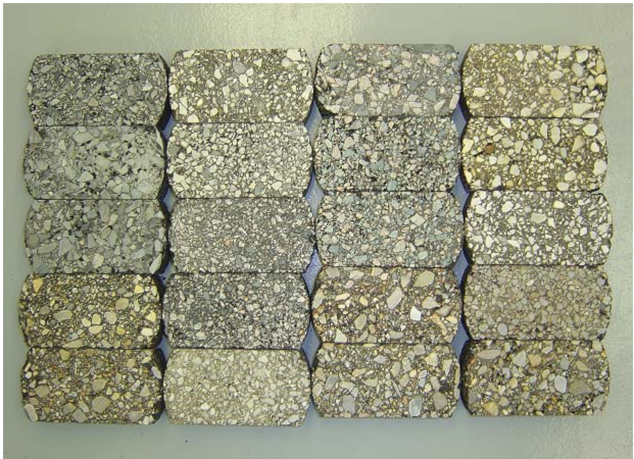
Figure 8. OT Specimens Cut from Double-Blade Saw.
