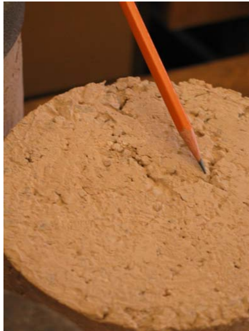
Figure 3. Surface Irregularities before Filling with Fines for TST Sample.
