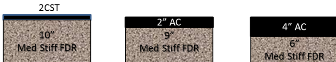
Figure 4. Comparison of Pavement Sections Using Table 5 for 4 Million ESAL, Medium Stiff Subgrade and Medium Stiff Stabilized FDR.
