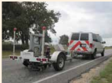
Figure 3. Falling Weight Deflectometer
