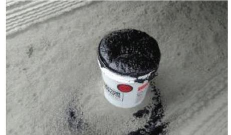
A test checking the expansion of foam asphalt.
