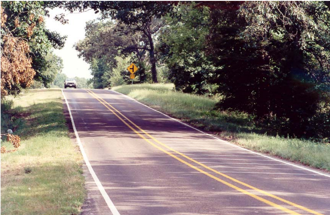
Figure 7-11. Grade Change Sight Distance Restriction.
