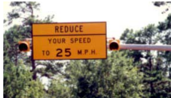
Figure 7-24. Flashers Activated When Speeds Exceed 30 MPH.
