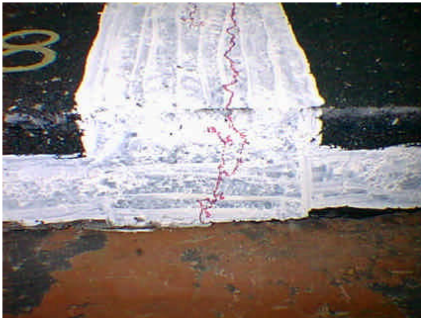
Figure 14. Sample Tested to Failure with Crack Locations and Load Cycles Indicated.
