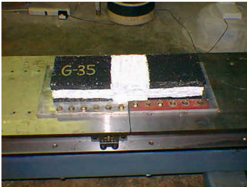
Figure 13. Beam Sample Epoxied to Aluminum Plates, Painted, and Bolted to the TTI Overlay Tester.
