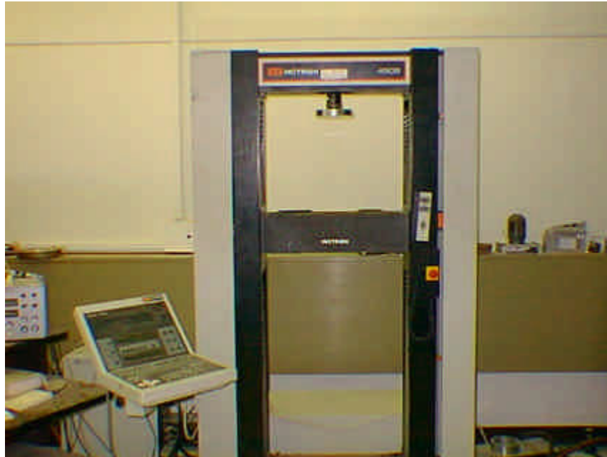
Figure 9. Instron 4505 Testing Machine with Instrument Panel Used to Apply 20,000-lb Leveling Load.
