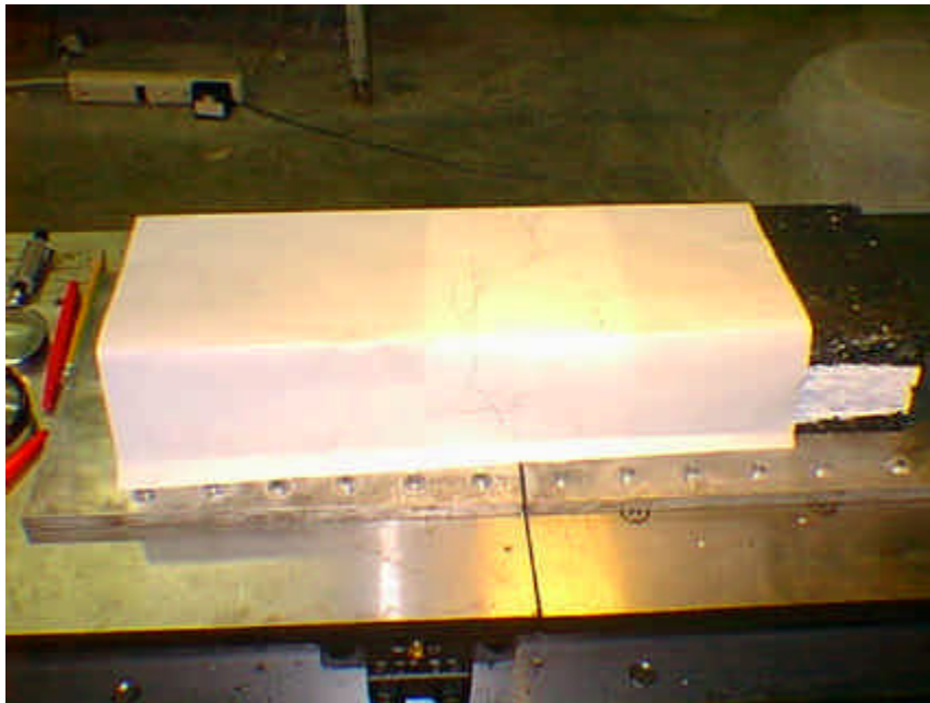
Figure 15. Tracing Paper Used to Record the Crack Patterns and Corresponding Load Cycles.
