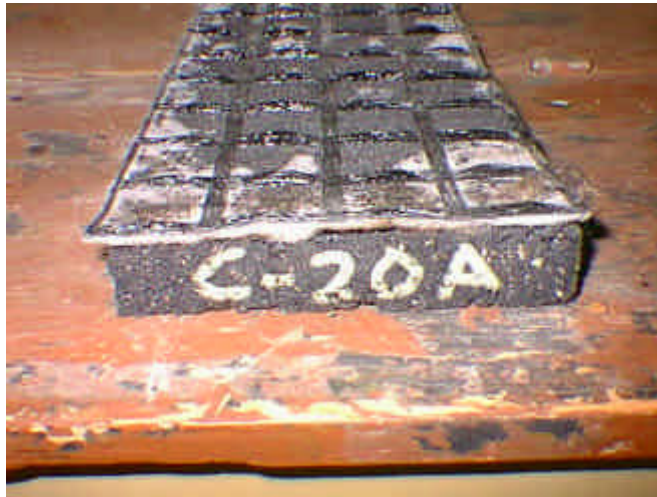
Figure 5. Uneven Coverage Using MS-1 Emulsified Asphalt Applied to Sample Beam C-20A with the HaTelit C40/17 Composite Product.
