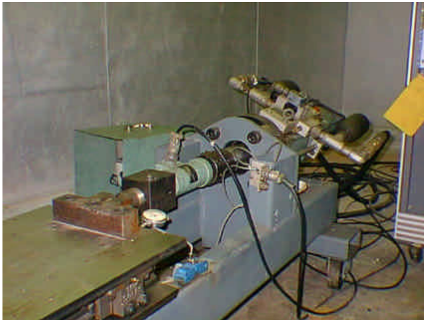
Figure 11. TTI Overlay Tester and Hydraulically Powered Ram Assembly. (Only the Movable Base Plate is Shown.)
