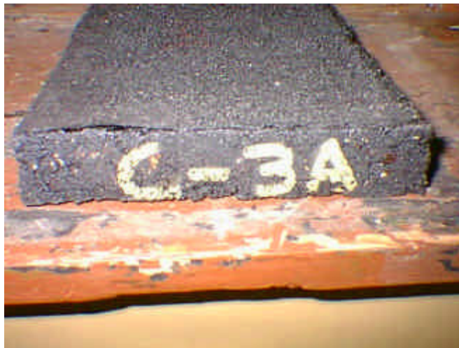
Figure 6. Lack of Complete Adhesion Using MS-1 Emulsified Asphalt Applied To Sample Beam C-3A with the Pave-Dry 381 Fabric.
