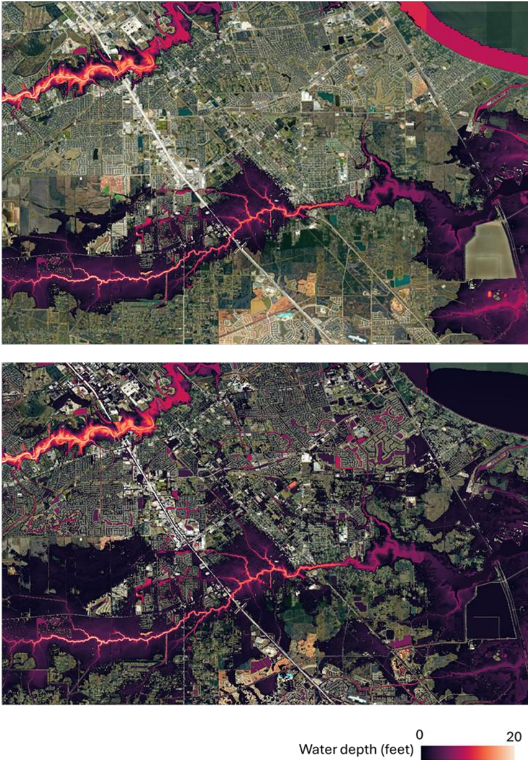
Figure 5. One-in-100-Year Flood Risks for Southeast Houston Shown as Flood Water Depth for Coastal Surge/River Overtopping (Upper) and Additional Pluvial Flooding Caused by Rainfall Intensities/Durations Exceeding Hydraulic Holding or Drainage Capacities (Lower).
