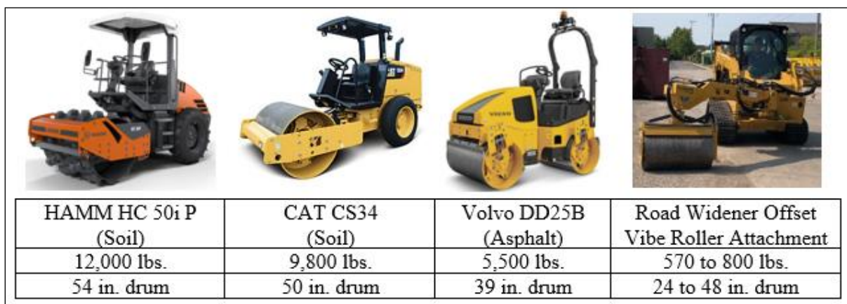
Figure 22. Example of Compactors for Narrow Widenings ( https://www.wirtgen-group.com/ , https://www.cat.com/ , https://www.volvoce.com/ ).
