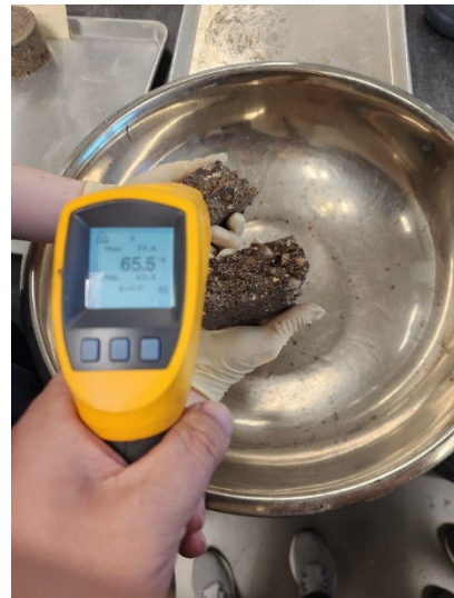
(d) After molding: internal temperature of specimen (65.5°C)
