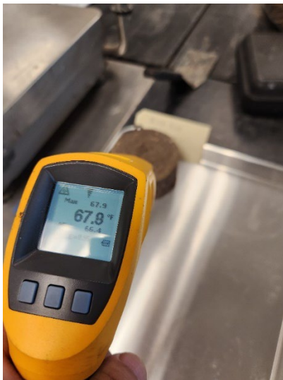
(c) Immediately after molding: surface temperature (67.8°C)
