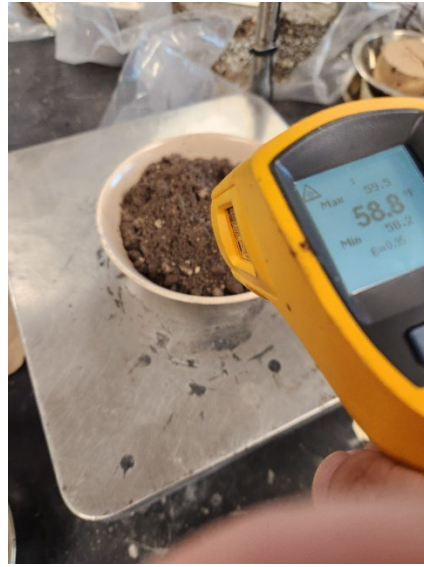
(b) Measured before molding: during material weighing (58.8°C)
