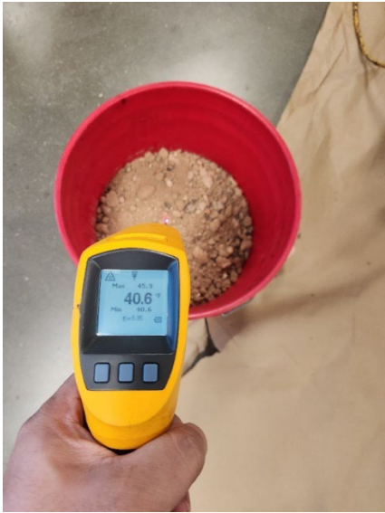
(a) After 24 hours of temperature conditioning of material (40.6°C)
