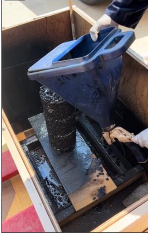
Figure 80. Cantabro specimens stacked rejuvenator application.
