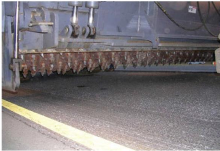
Figure 18. Micromilling equipment teeth (Jared and Hines 2014).
