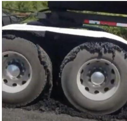
Figure 14. PFC pavement surfaced with AR seal coat tracking on vehicle tires immediately after construction.
