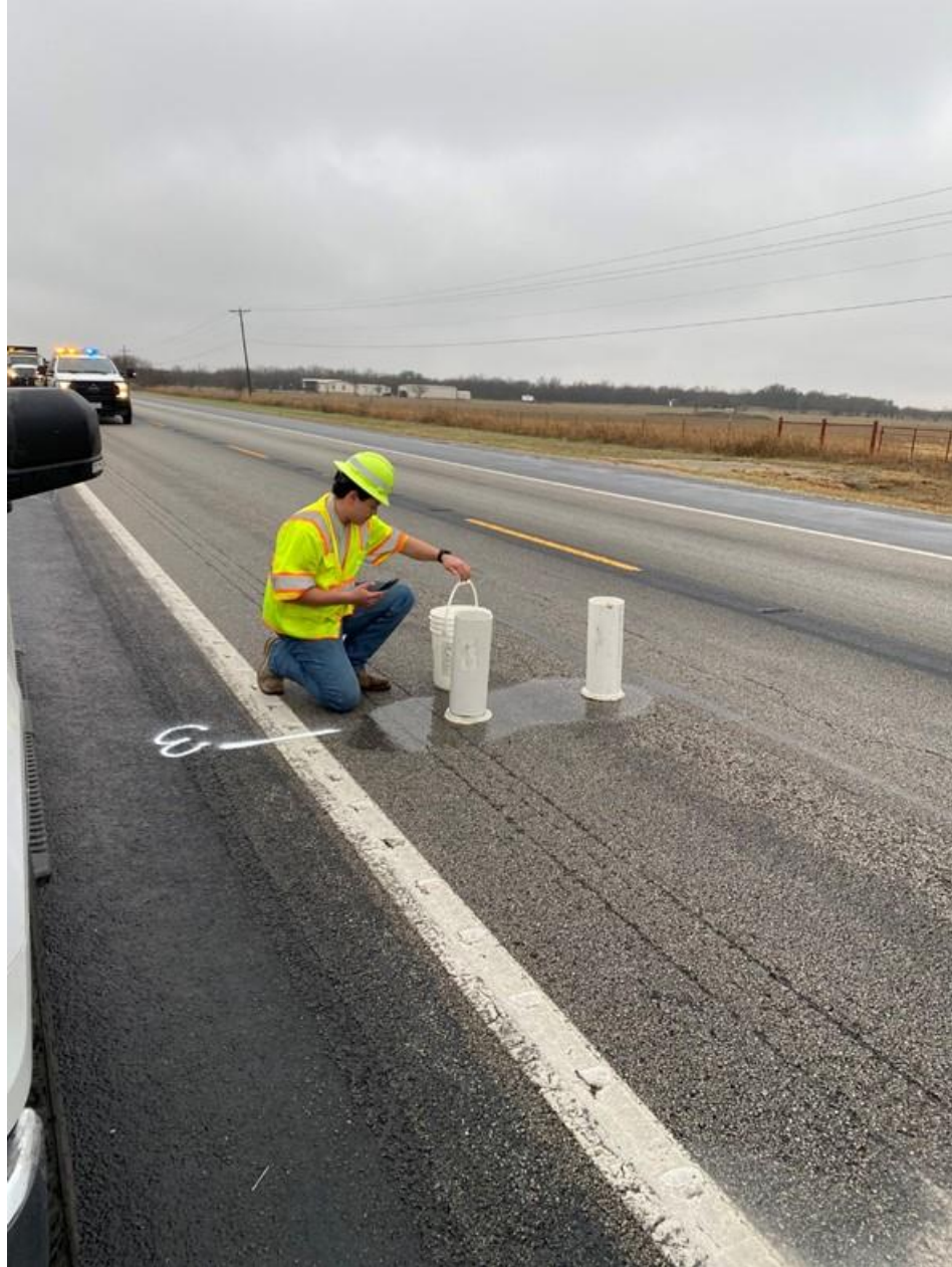
Figure 71. Water flow testing.
