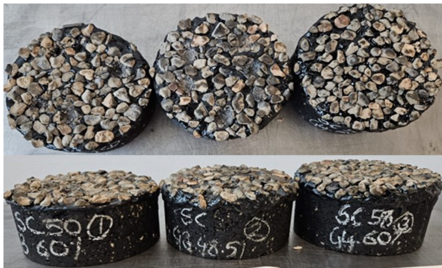
Figure 3. Laboratory Seal Coat Specimens with 1, 2, and 3 Layers.
