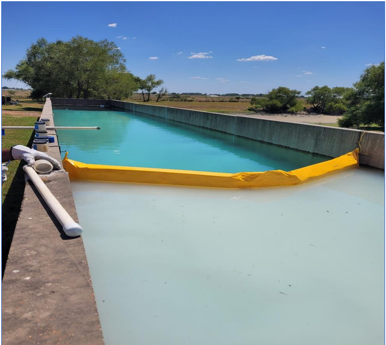
Figure 11. Floating Turbidity Barrier Evaluation Test System.
