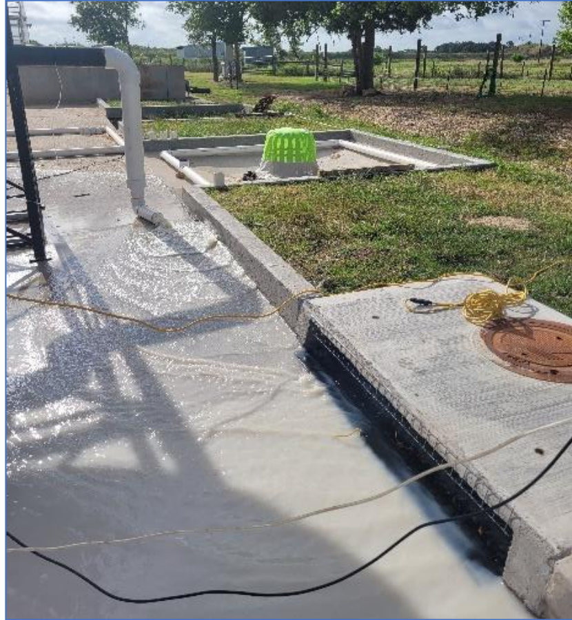
Figure 6. Curb/Gutter Protection Evaluation Test System.
