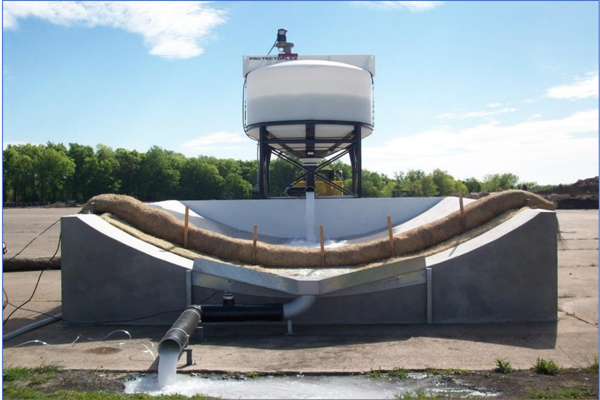
Figure 9. Channel/Perimeter Protection Evaluation Test System.
