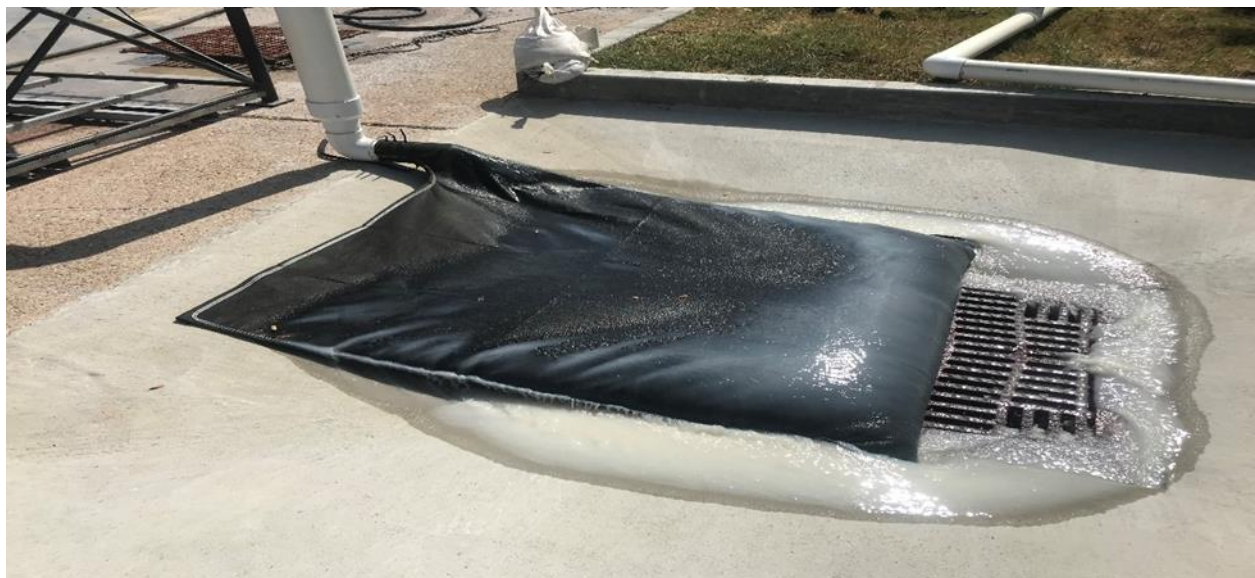
Figure 10. Geotextile Dewatering Device Evaluation Test System.
