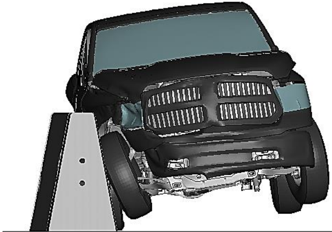
b. t = 0.35 s, event = rear right tire contacts the barrier
