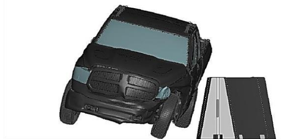
c. t = 0.54 s, event = vehicle stabilizes post impact
