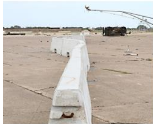
b. Test article after impact
