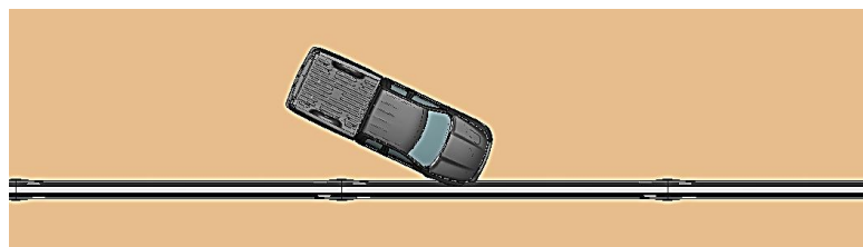
a. t = 0.17 s, event = pickup truck strikes the barrier
