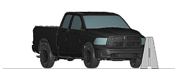
a. t = 0.10 s, event = front right tire contacts the barrier
