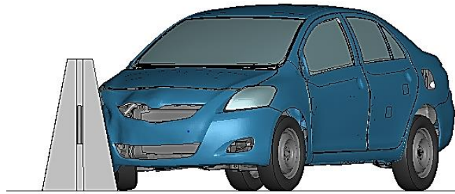
a. t = 0.19 s, event = passenger car impacts barrier
