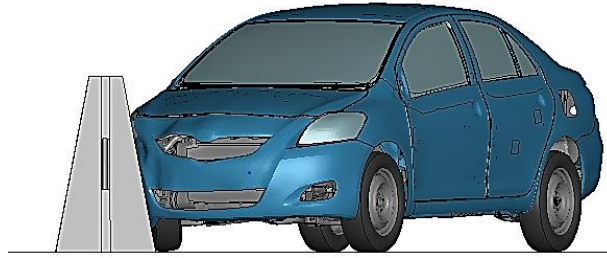
a. t = 0.19 s, event = passenger car contacts barrier
