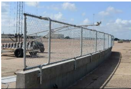
Figure 2.3. TxDOT Chain-Link Fence Supported by Weak Post prior to Testing.
