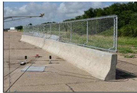
Figure 2.3. TxDOT Chain-Link Fence Supported by Weak Post prior to Testing.
