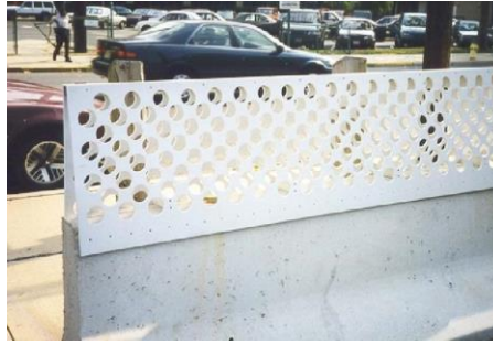
Figure 2.9. Prototype of Side-Mount CGSPF Using Recycled Plastics (8).
