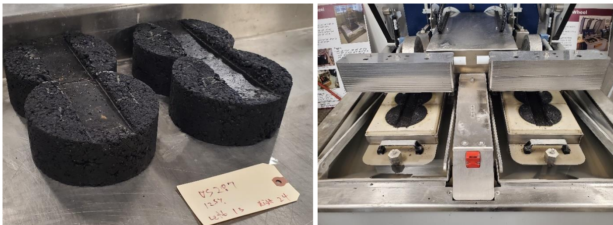
Figure 77. Example Hamburg Test (Tex-242-F).
