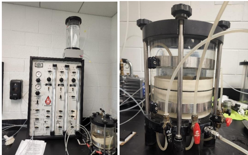
Figure 81. Permeability Test (ASTM D 5084).
