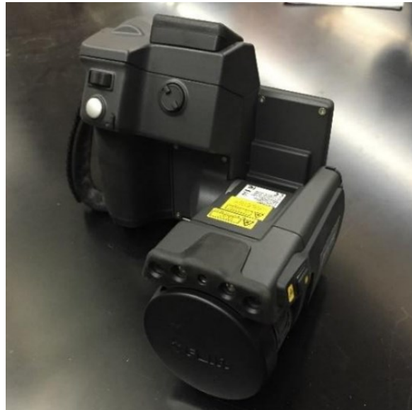
Figure 2.4. FLIR T640 Infrared Camera for IRT Inspection.
