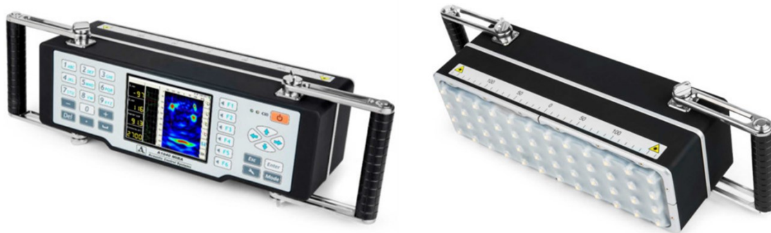
Figure 2.6. MIRA A1040 for UST Inspection.
