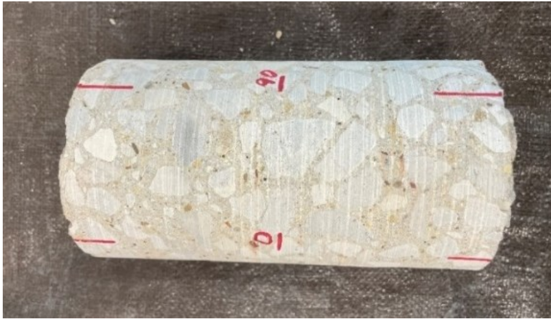
Figure 4.3. Concrete Core Specimen with Marks at 0 and 90 Degrees.
