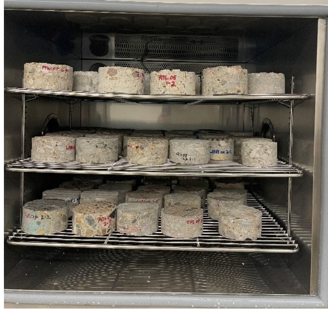
Figure 4.17. Concrete Samples inside Environment Chamber.
