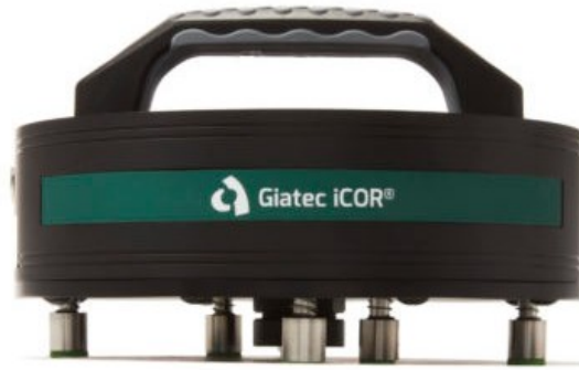
Figure 2.8. Giatec iCOR Used for Corrosion Rate Mapping Inspection (Giatec, 2019).
