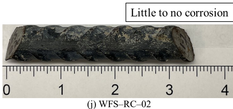
Figure 4.45. Extracted Black Rebar from Concrete Core Specimens (Cont.).
