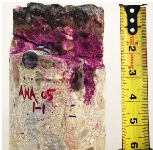
Figure 4.31. Measurement of Carbonation Depth for Concrete Specimens.
