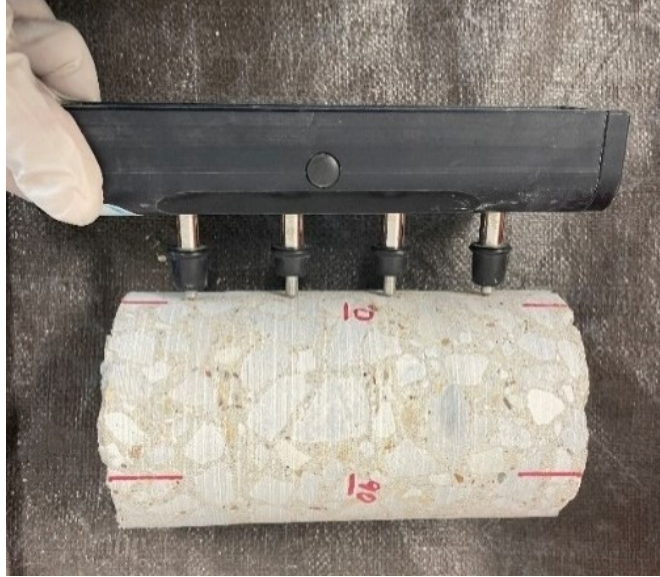
Figure 4.2. Measurement of Surface Resistivity Using 4-point Wenner Array Probe.
