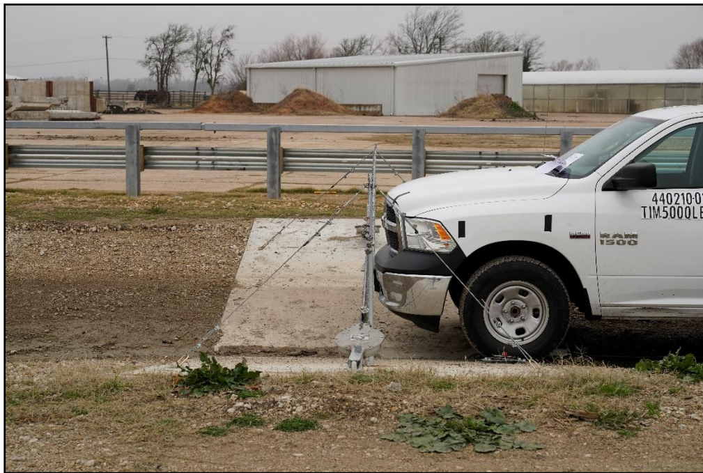
Figure 9.2. MOPS/Test Vehicle Impact Location for Test 440210-01-4.
