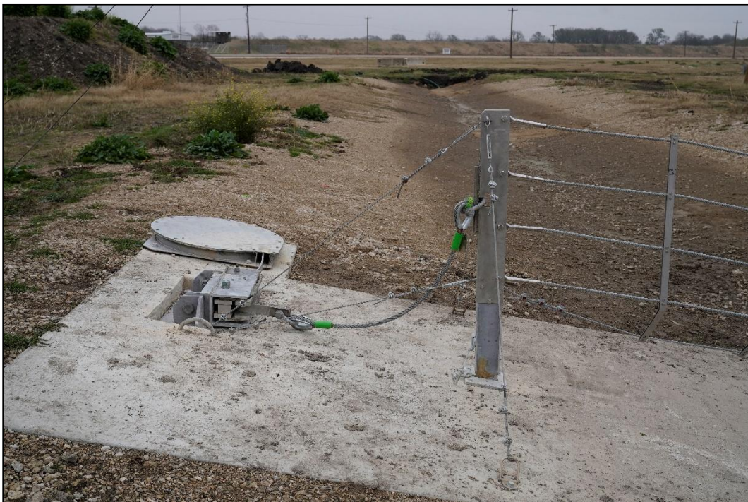
Figure 4.11. Anchor Hardware for the Second Median Opening Protection System Net prior to Crash Tests 440210-01-4, 440211-01-3, 440211-01-5, and 440213-01-6.
