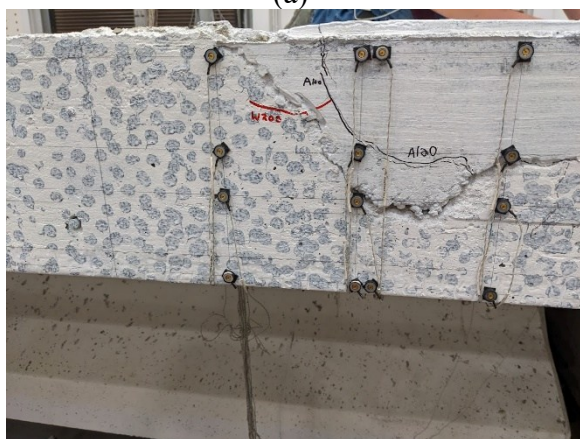
Figure 9.54. PBJ-OP1R—north overhang of HPC retrofit region: (a) diagonal cracks formed at west end during loading to 20 kips of Pattern All-1; (b) west end after all loading; (c) east end after all loading; and (d) shallow vertical cracks at center of slab after all loading.
