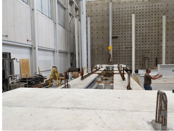
Figure 9.25. Girders in place for PBJ-OP1 deck construction (far ends of the girders have the deck from the PBJ-FP1R test).
