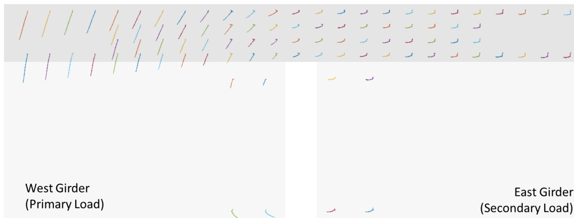
Figure 10.21. PBJ-FP1: Optotrak target displacement history for Pattern W.
