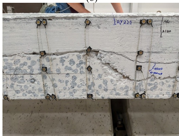
Figure 9.54. PBJ-OP1R—north overhang of HPC retrofit region: (a) diagonal cracks formed at west end during loading to 20 kips of Pattern All-1; (b) west end after all loading; (c) east end after all loading; and (d) shallow vertical cracks at center of slab after all loading.
