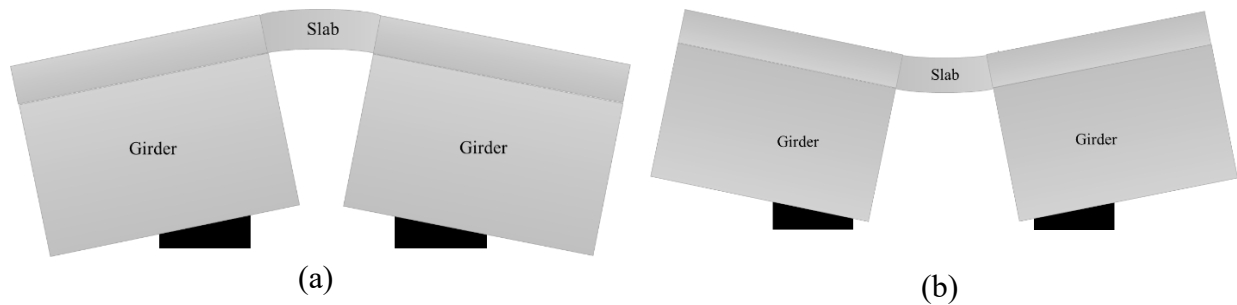
Figure 9.1. Sign convention used for discussion of continuous deck demands: (a) positive bending and (b) negative bending.
