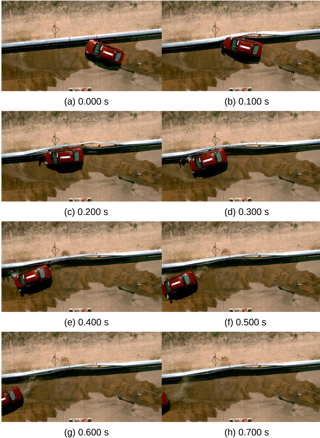
Figure C.4. Sequential Photographs for Test 469940-03-1 (Overhead Views).
