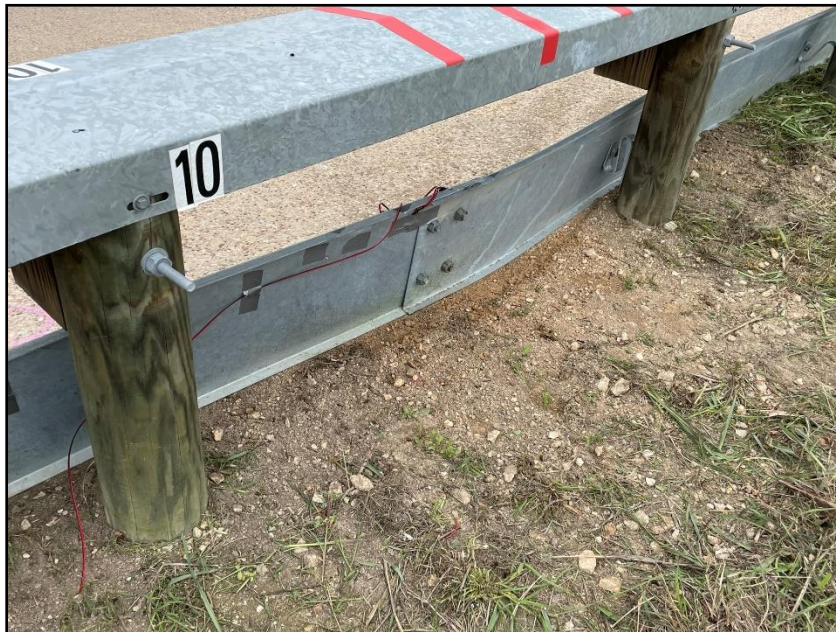
Figure 17.4. Field Side of the Enhanced Motorcycle Guard Fence System at Impact Location after Test 469943-01-2.
