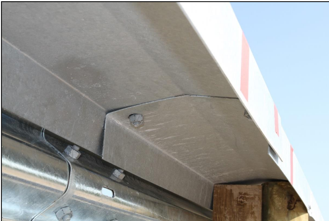
Figure 6.7. Enhanced Motorcycle Guard Fence System Cap Rail Hardware Detail prior to Testing for 469940-03-1, 469940-03-2, 469940-03-3, and 469940-03-4A.
