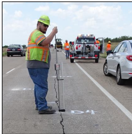
Figure 18. Dynamic Cone Penetrometer Testing.
