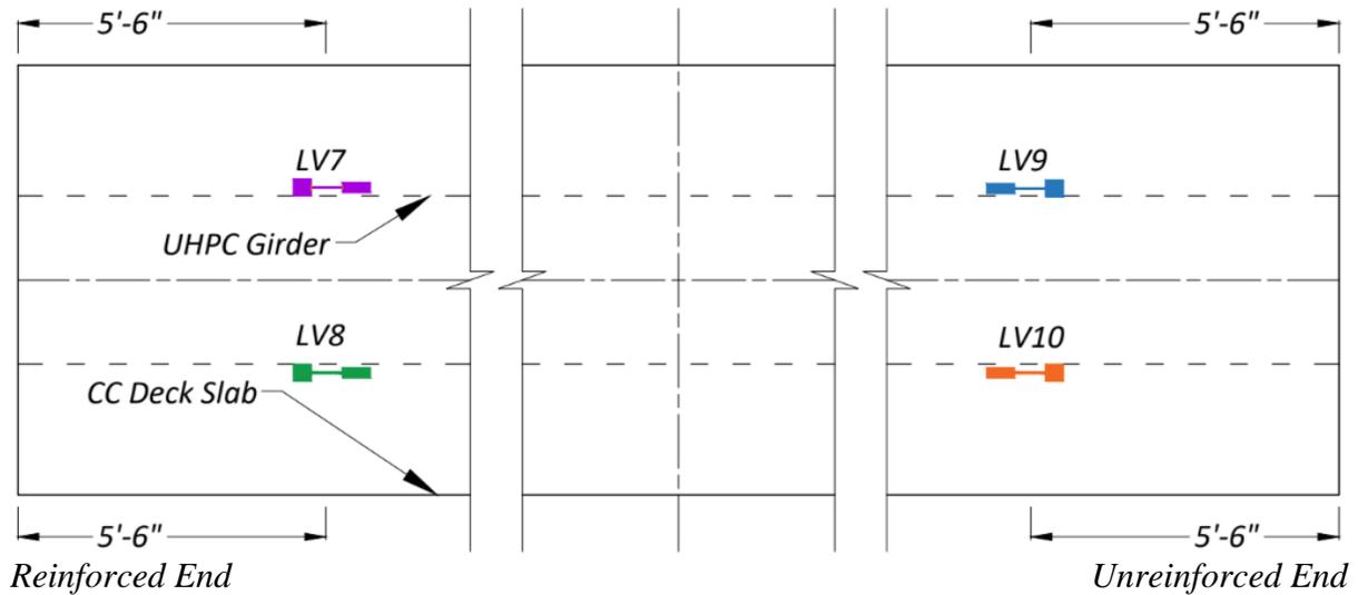
(a) Layout of LVDTs Measuring Interface Slip
