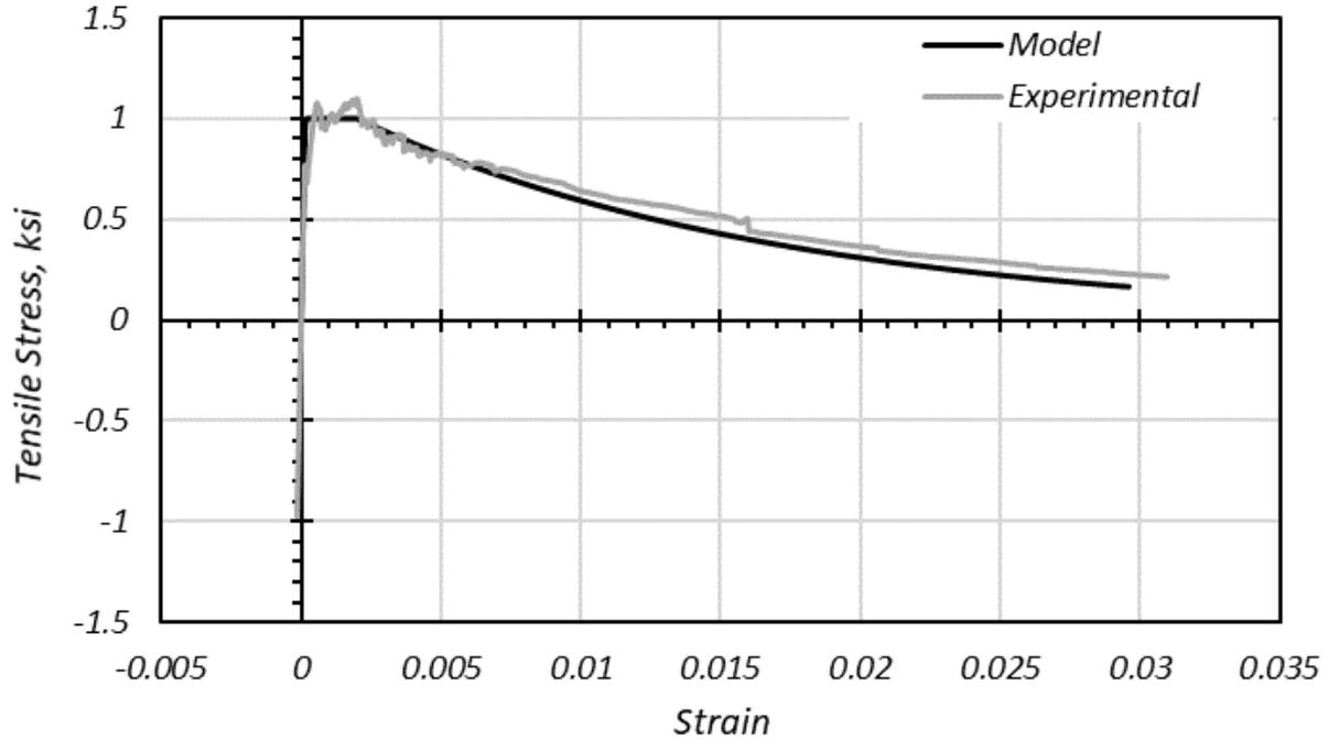
**Figure 5.10. Uniaxial Tension Test: Experimental Data versus Model.**
