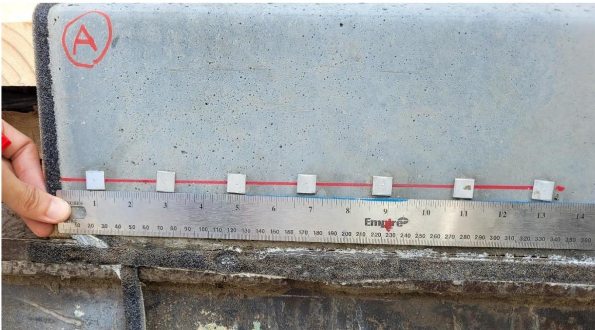
(b) Attached Aluminum DEMEC Points on Tx34-2
