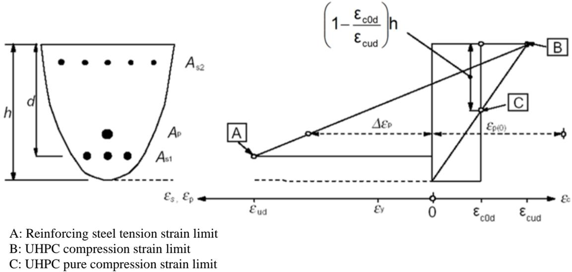
**Figure 2.10. Stress-Strain Distribution in Cross-Section (NF-P-18-710 2016).**
