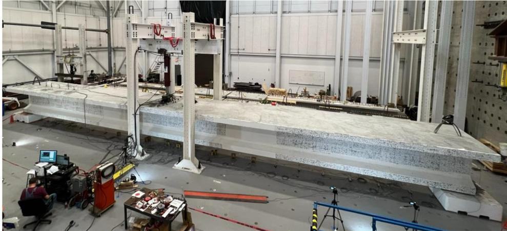
*(a) Tx54 Test Setup (Overhead View)*
