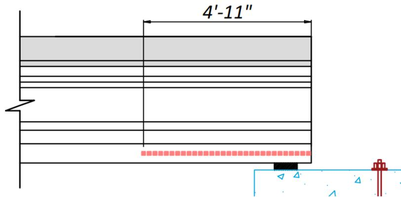
(a) Tx34-1 – 30 DEMEC Points at 2 in. Spacing
