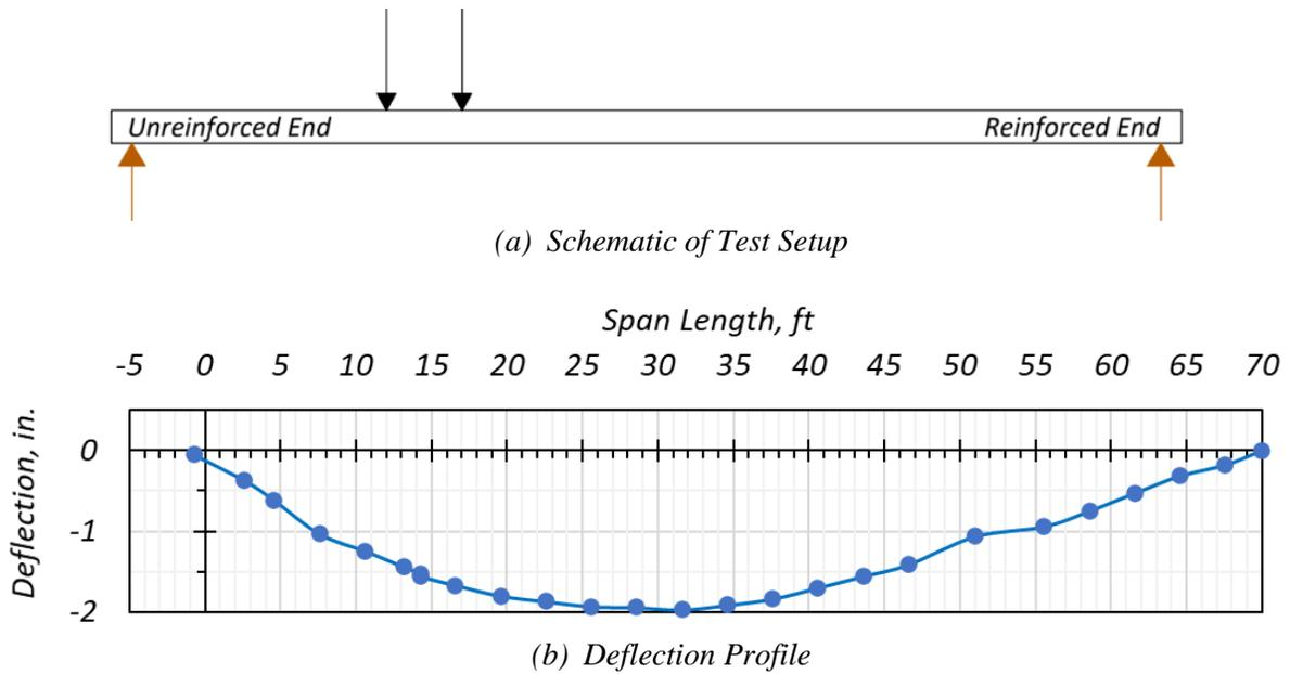
**Figure 6.62. Tx54 Shear Test 2: Deflection Profile.**
