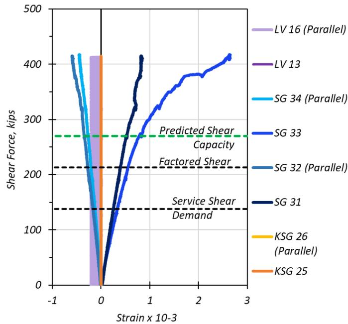
**Figure 6.22. Tx34-1 Shear Test 2: Web Strains (Reinforced End).**
