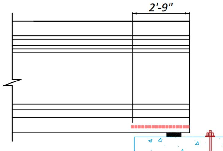
(c) Tx54 – 9 DEMEC Points at 4 in. Spacing
