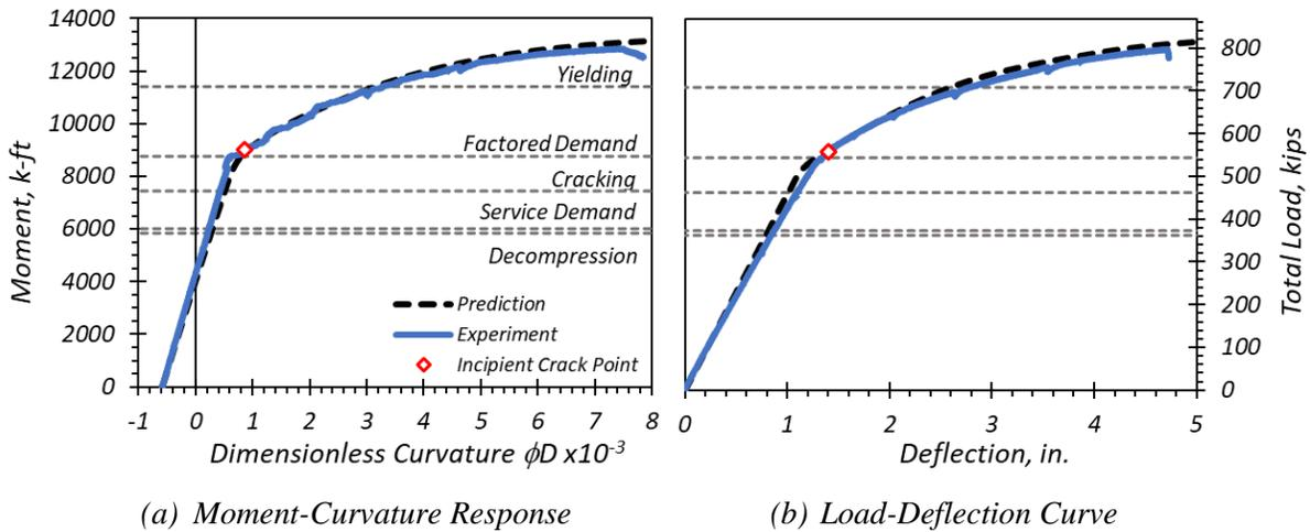
**Figure 5.30. Tx54 Flexure Test Response.**
