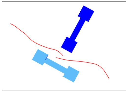
**Figure 4.14. SGs in Web at Shear Cracks.**
