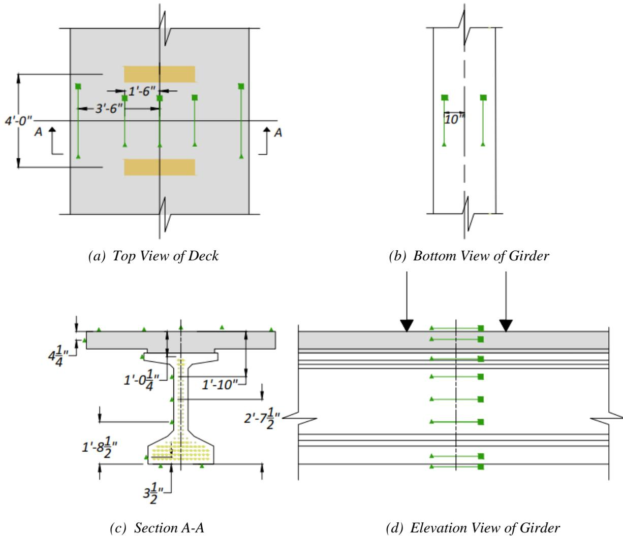
**Figure 4.10. Tx54-2 SPs between Actuators at Midspan.**
