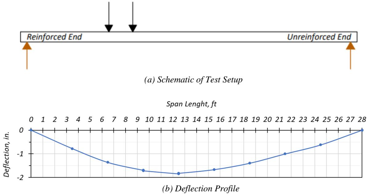
**Figure 6.44. Tx34-2 Shear Test 2: Deflection Profile.**
