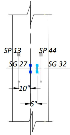
(b) Underside of UHPC girder soffit
