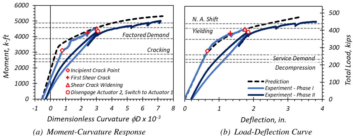
Note: Phase I loading and unloading (light blue) is followed by Phase II loading (dark blue).
