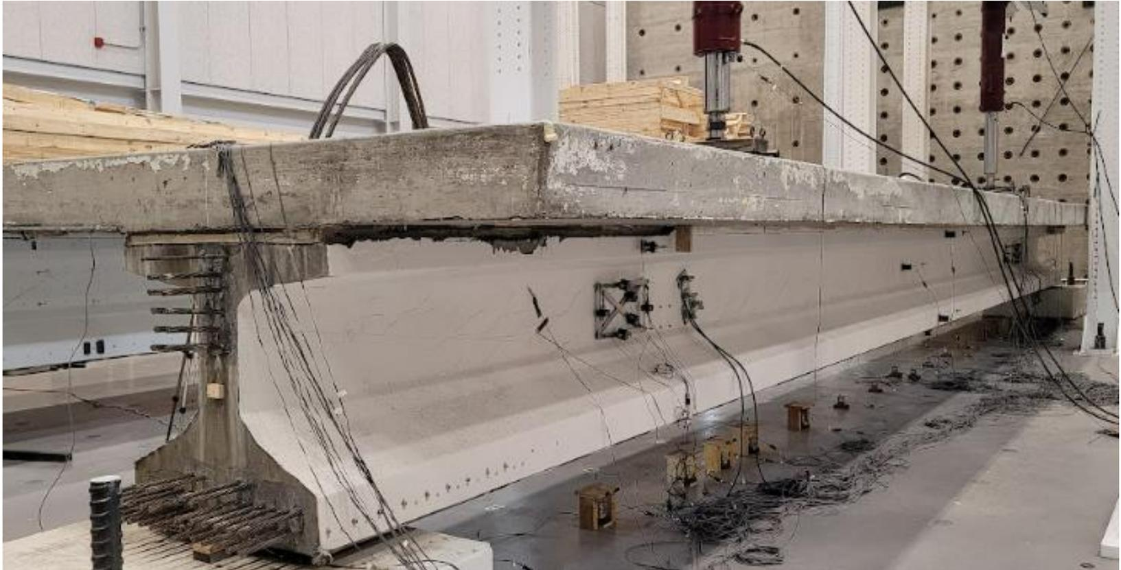
**Figure 6.4. Tx34-2 Test Setup and Instrumentation for Shear Test 1 (North Face).**
