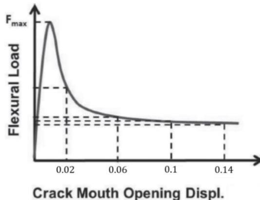
**Figure 2.16. Schematics of a Typical Test Result (EN 14651 2005).**
