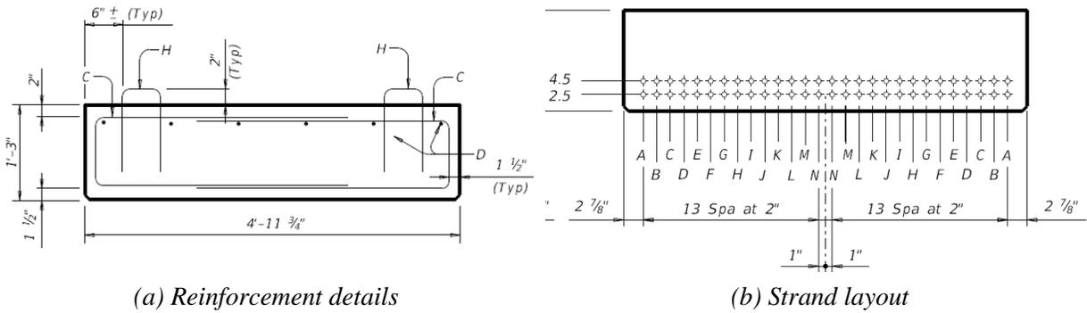
**Figure 3.3. Section Geometry of 5SB15 Slab Beam.**
