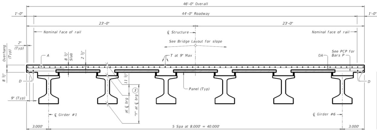
**Figure 3.15. Typical Bridge Cross-Section Using Tx54 Girders (TxDOT 2019).**
