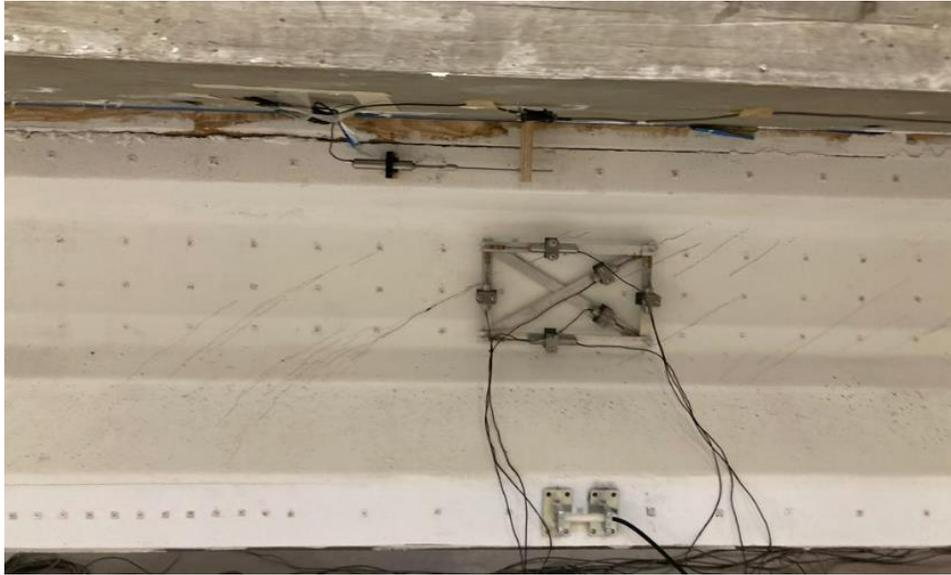
**Figure 5.16. Tx34-1 Shear Cracks at Unreinforced End at 450 Kips.**
