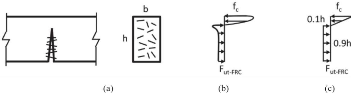
**Figure 2.15. Schematics of Stress Block for a Cracked FRC Flexural Member: (a) Beam Section, (b) Actual Distribution of Normal Stresses, (c) Simplified Distribution of Normal Stresses (ACI 544.4R-18 2018).**
