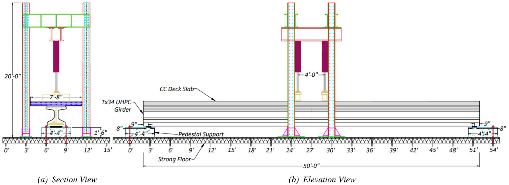
**Figure 5.1. Flexure Test Setup for Tx34-1 and Tx34-2 Girder Specimens.**
