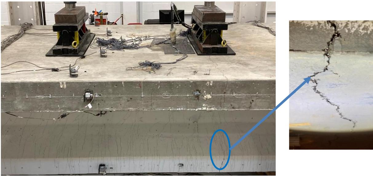
*(a) Cracks Formed at Midspan*
