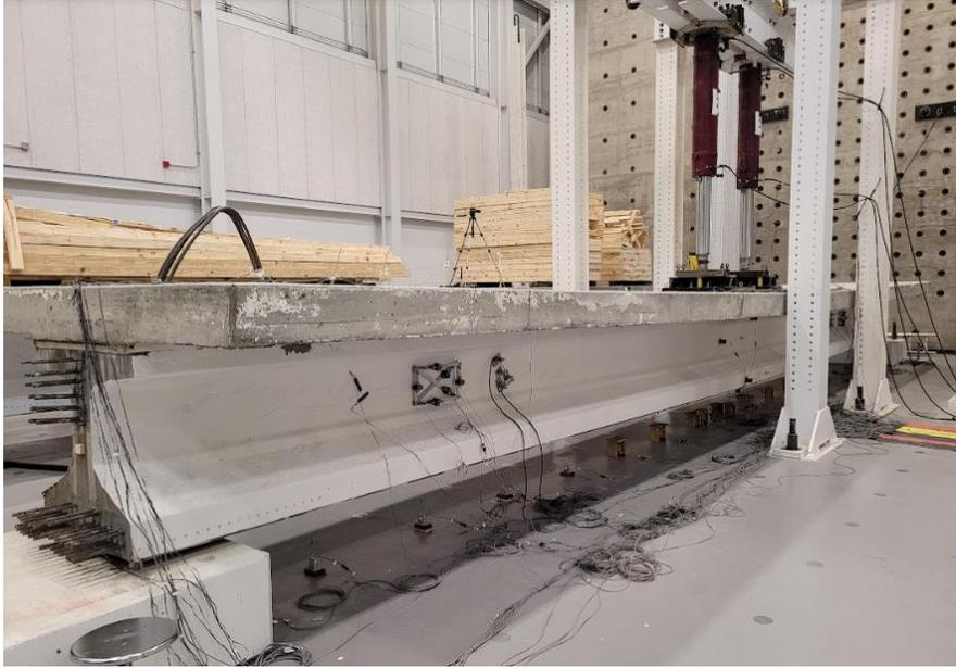
*(a) Tx34-2 Test Setup (North Elevation)*
