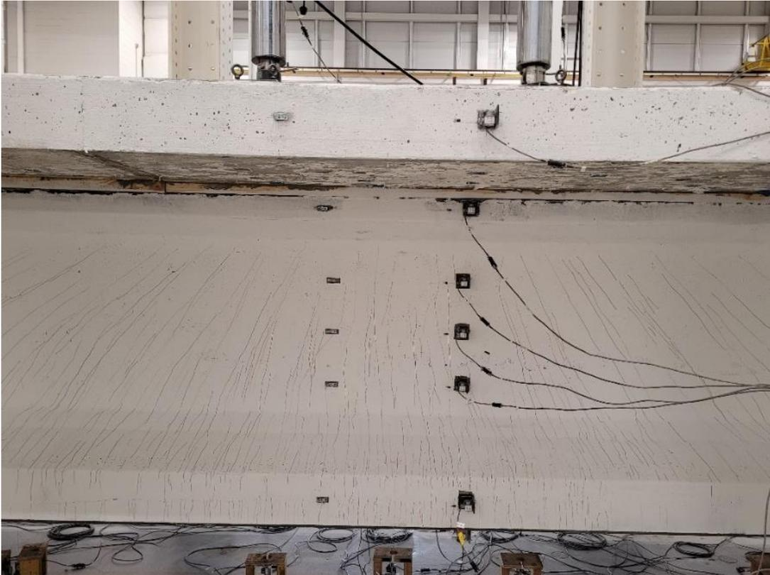
**Figure 5.33. Cracks in Constant Bending Moment Region Tx54.**
