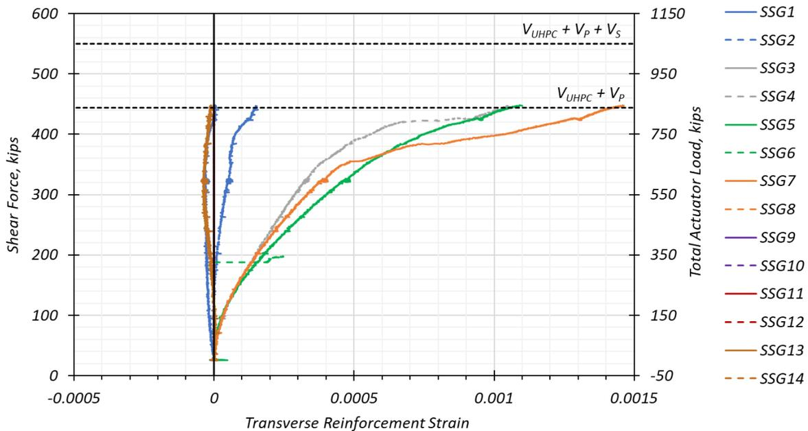
**Figure 6.30. Tx34-2 Shear Test 1: Transverse Reinforcement Strain Gages.**
