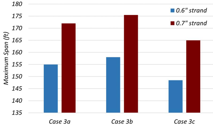
**Figure 3.30. Comparison of Maximum Span Lengths for UHPC Tx54 Girders.**
