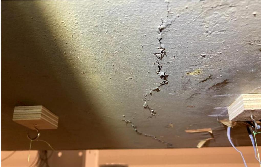
**Figure 5.25. Fibers Bridging the Crack at the Underside of the Soffit of Tx34-2.**
