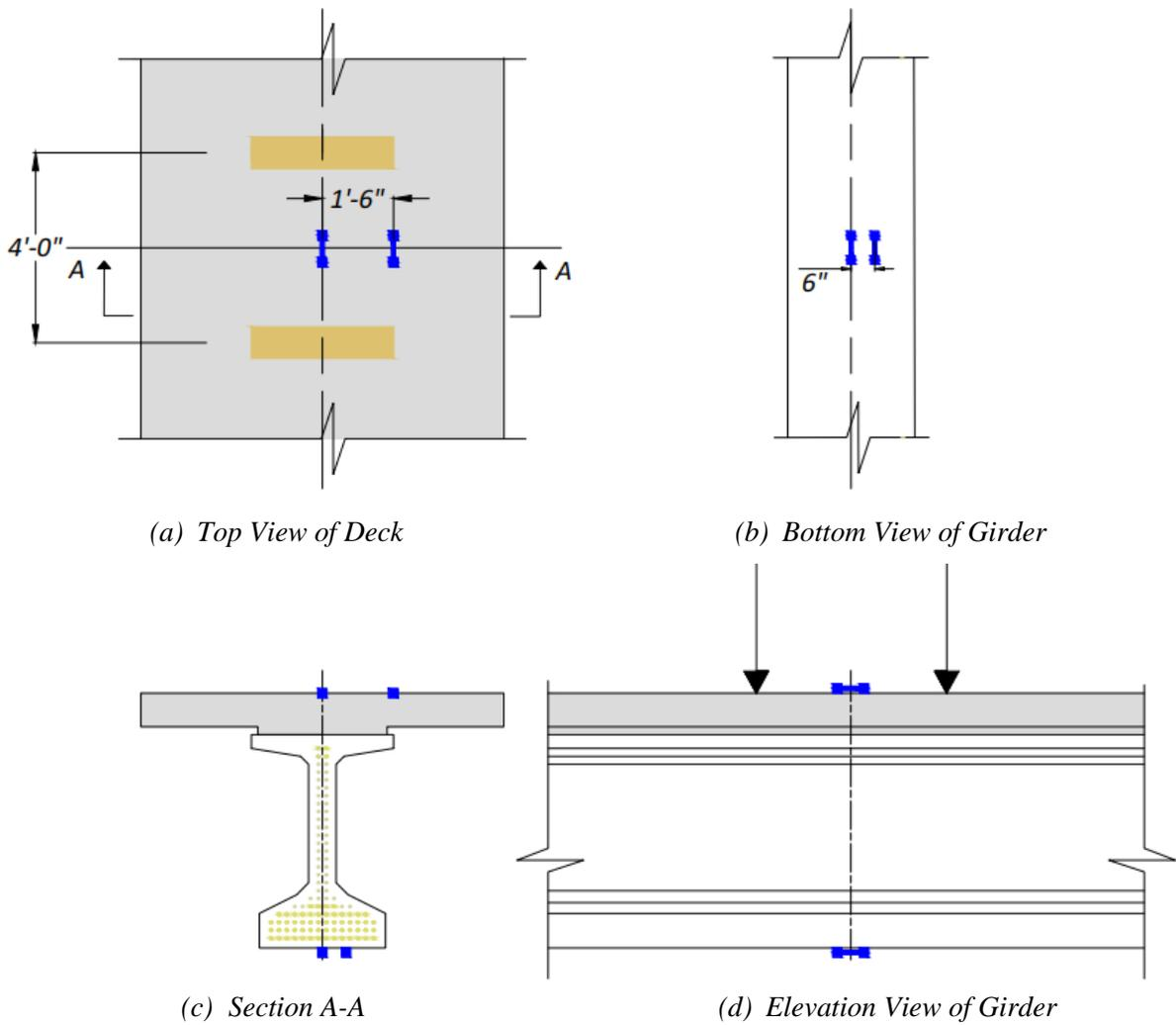
**Figure 4.13. Tx54 SGs between Actuators.**
