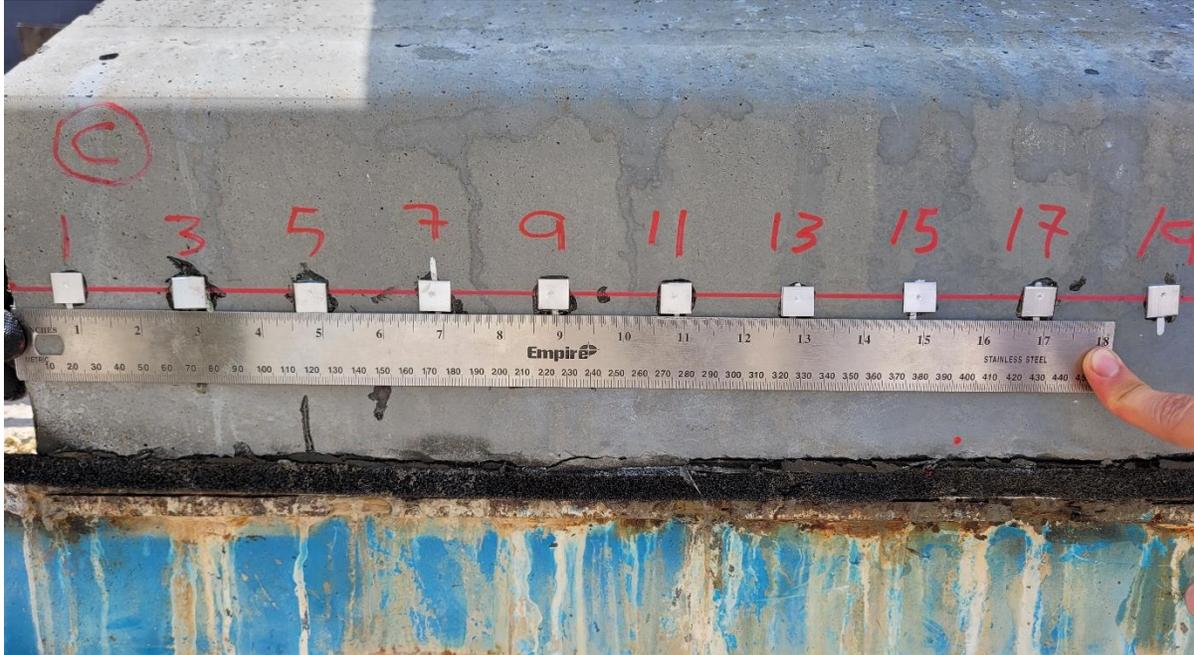
(a) Attached Aluminum DEMEC Points on Tx34-1
