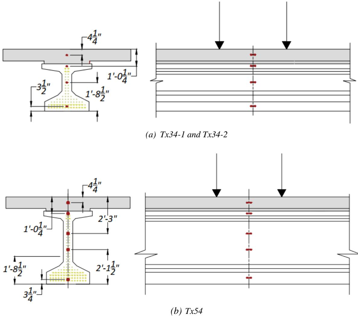
**Figure 4.16. Tx54 ESGs at Midspan.**
