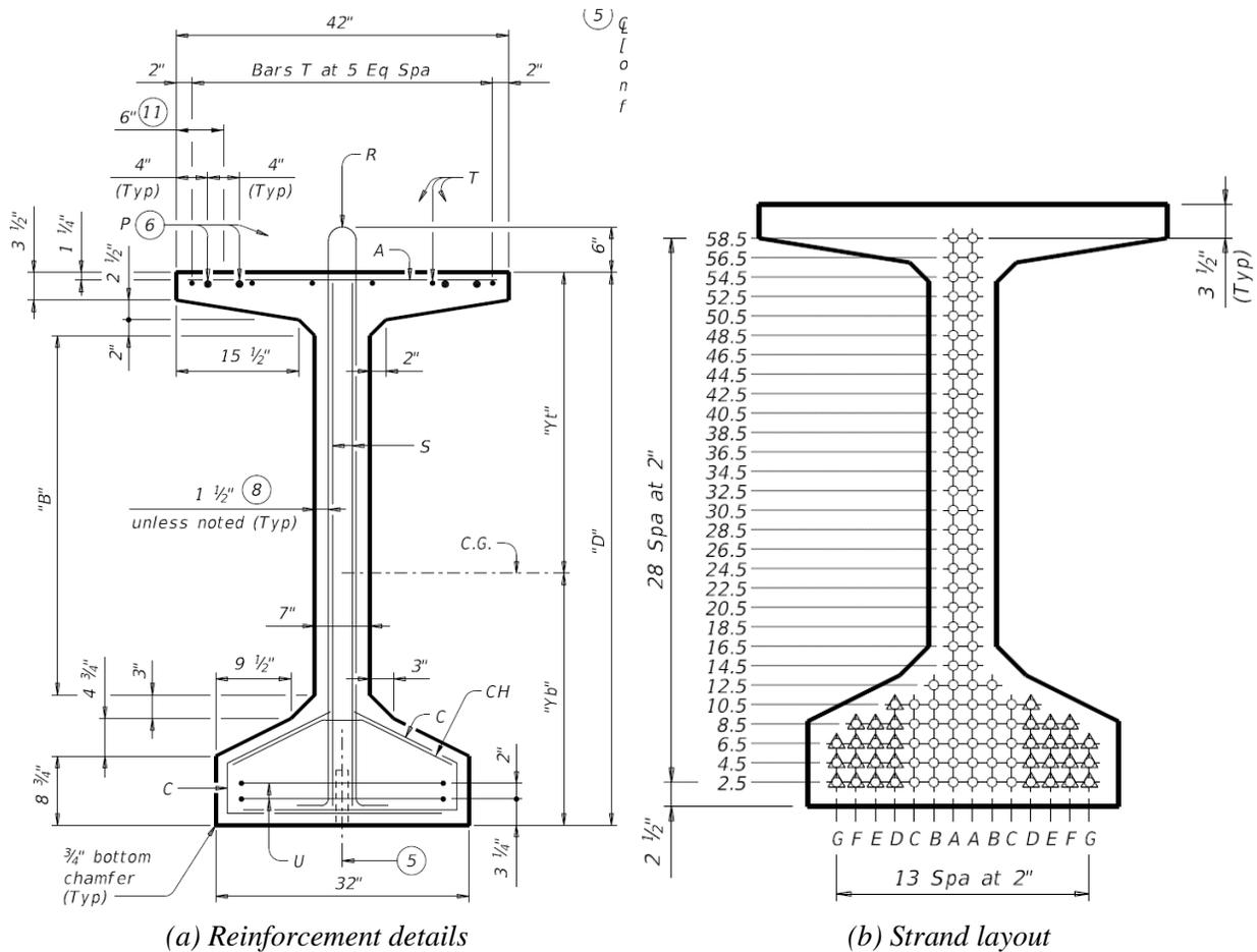
**Figure 3.34. Section Geometry of Tx62 I-Girder (TxDOT 2019).**
