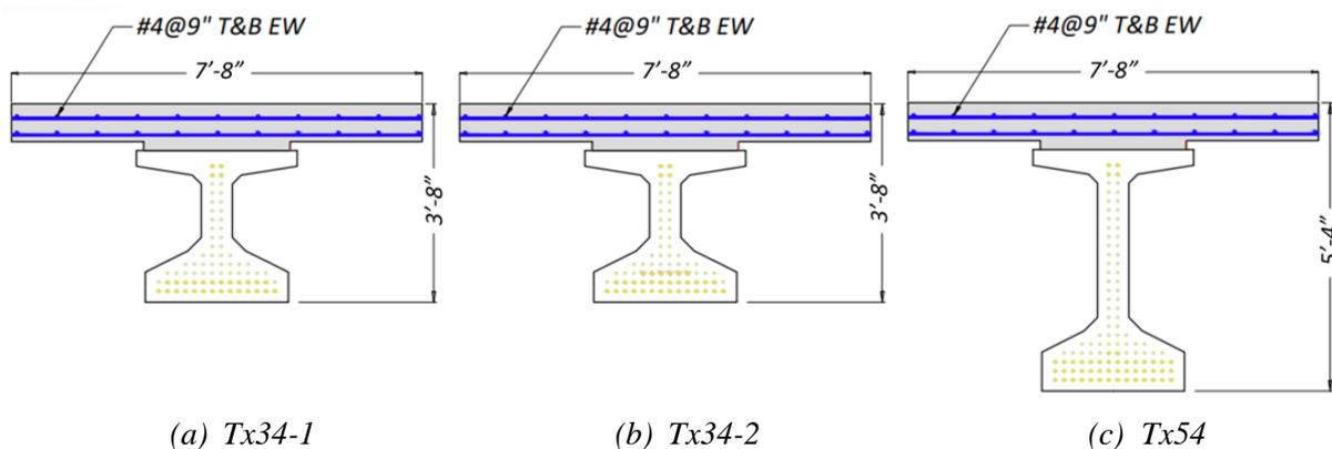
**Figure 4.4. CC CIP Deck Slab with UHPC Girders.**
