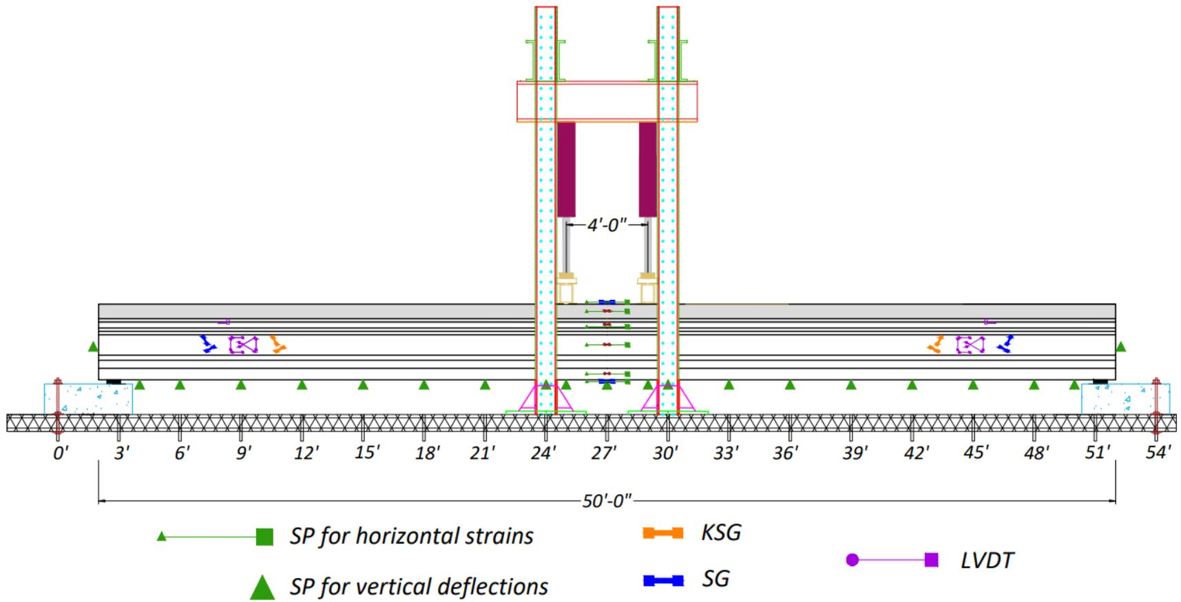
**Figure 5.7. Instrumentation for Flexure Test of Tx34-2.**
