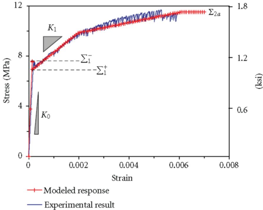
**Figure 2.12. Comparison of Modeled Response versus Experimental Response (Gunes et al. 2012).**
