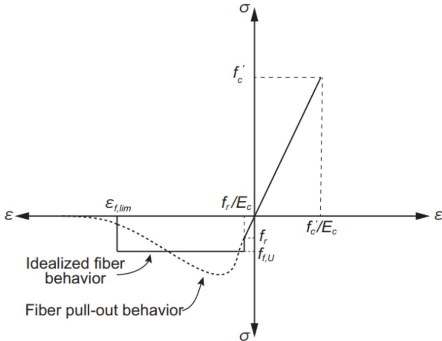
**Figure 2.13. Assumed UHPC Behavior (Giesler et al. 2018).**
