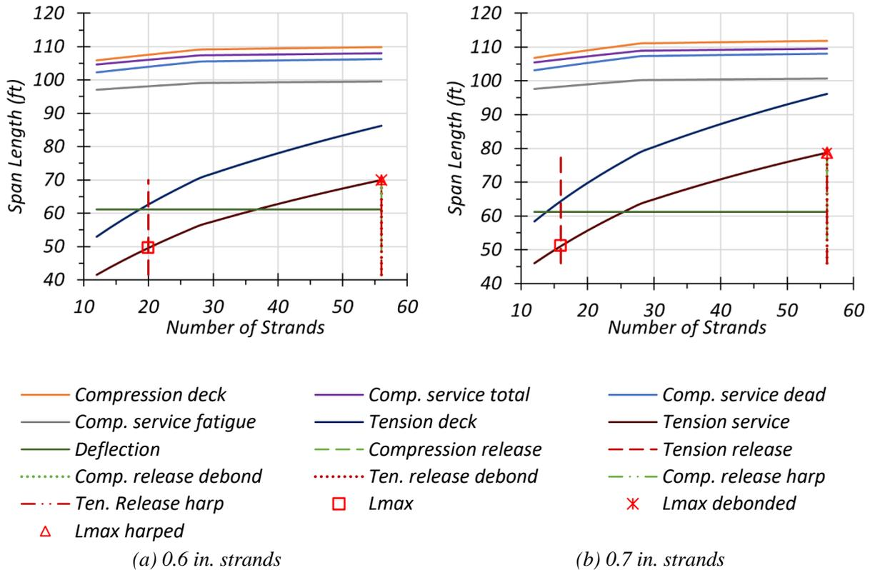
Note: Solid lines = maximum span, dashed lines = maximum number of strands.
