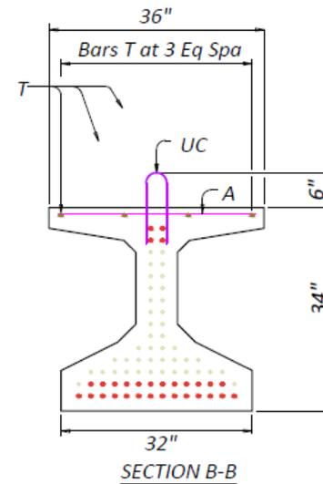
Note: Thermocouple (TC) and Embedded Strain Gage (ESG) are the sensors installed in the field.
