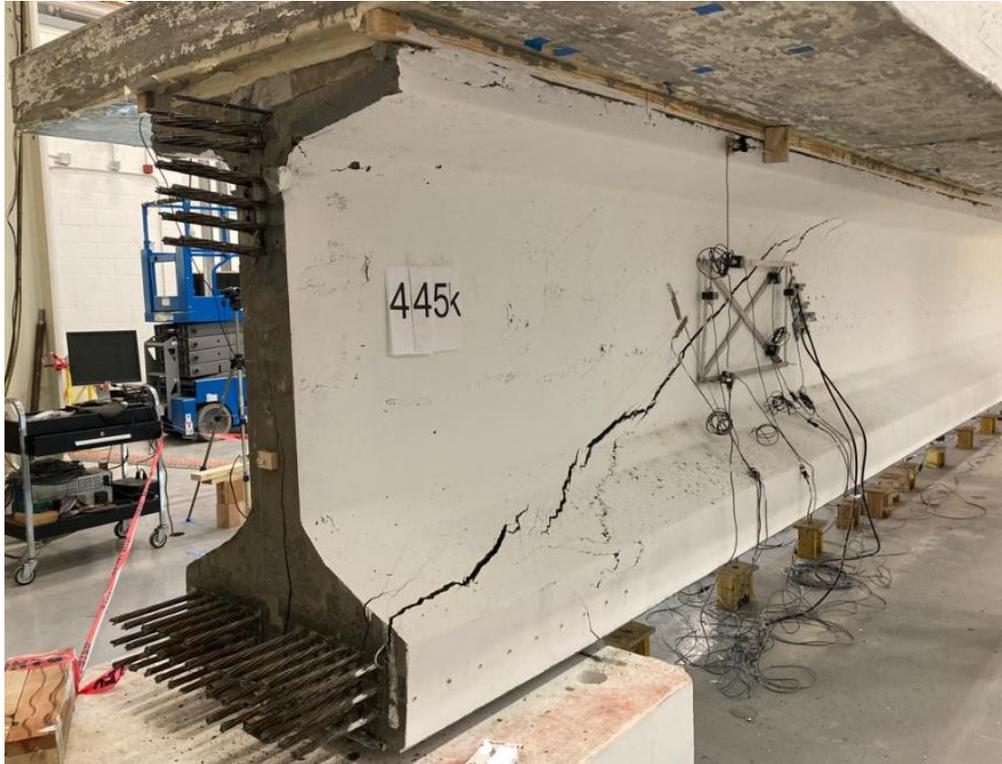
**Figure 6.55. Tx54 Shear Test 2: Shear Span of Unreinforced End at Failure.**
