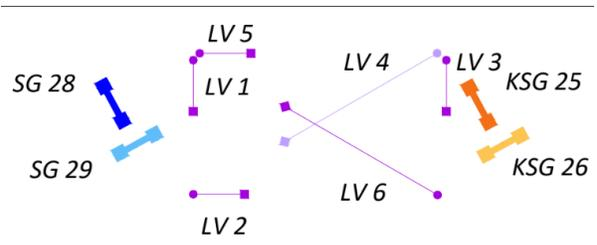
(b) Instrumentation Schematic of Shear End
