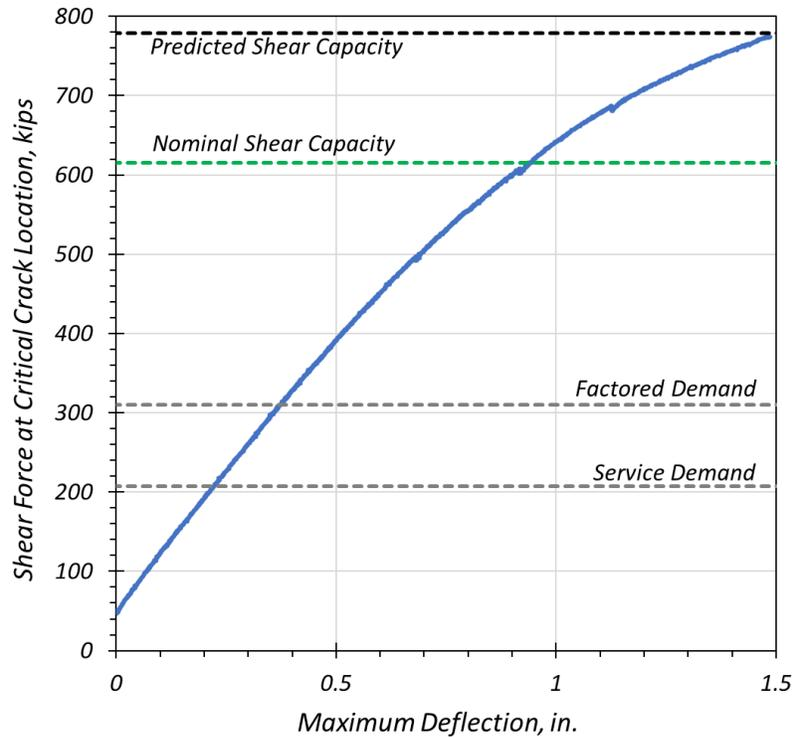
**Figure 6.50. Tx54 Shear Test 1: Shear Force versus Maximum Deflection (Reinforced End).**
