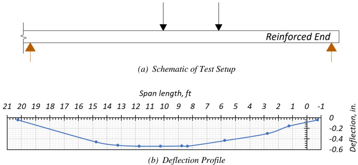
**Figure 6.26. Tx34-1 Shear Test 2: Deflection Profile.**
