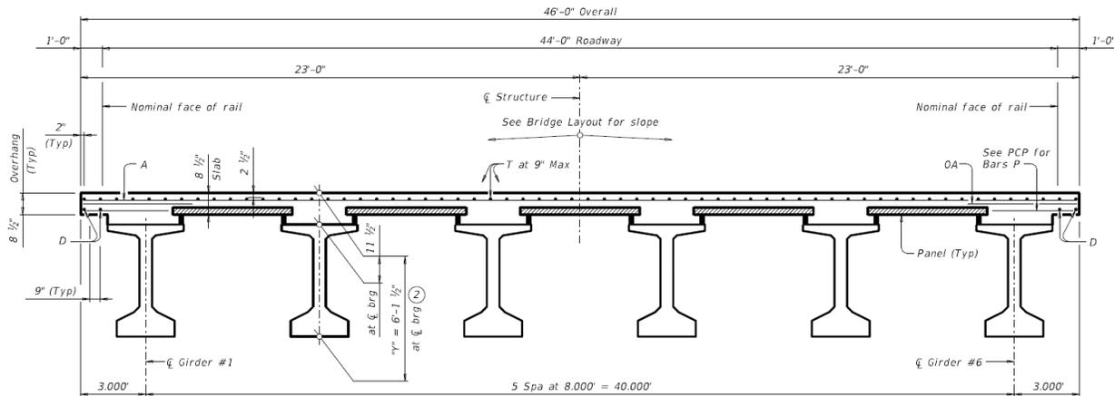
**Figure 3.33. Typical Bridge Cross-Section Using Tx62 I-Girders (TxDOT 2019).**
