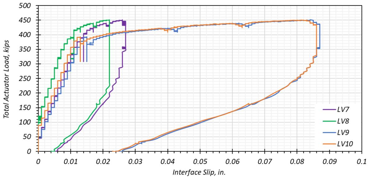
(b) Interface Slip During Phase II Testing
