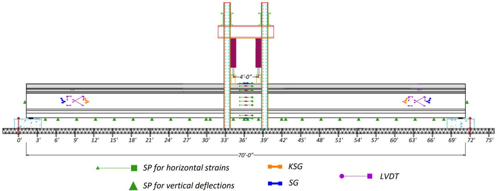
**Figure 5.8. Instrumentation for Flexure Test of Tx54.**
