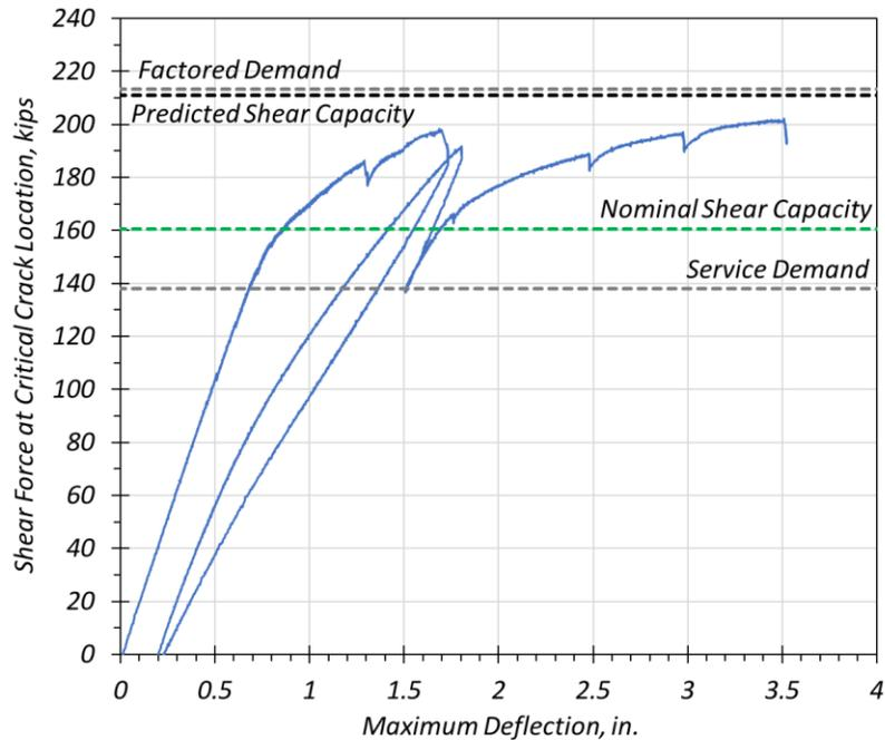
**Figure 6.16. Tx34-1 Shear Test 1: Shear Force versus Maximum Deflection (Unreinforced End at Termination of Phase II Flexure Test).**
