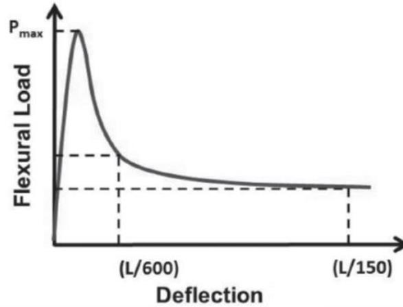
**Figure 2.14. Schematics of a Typical Test Result (ASTM C1609/C1609M 2012).**
