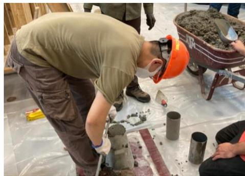
*Slump Testing and Sample Preparation*
