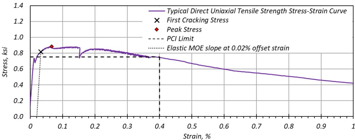
**Figure 4.21. Typical Uniaxial Tensile Strength Stress-Strain Curve.**
