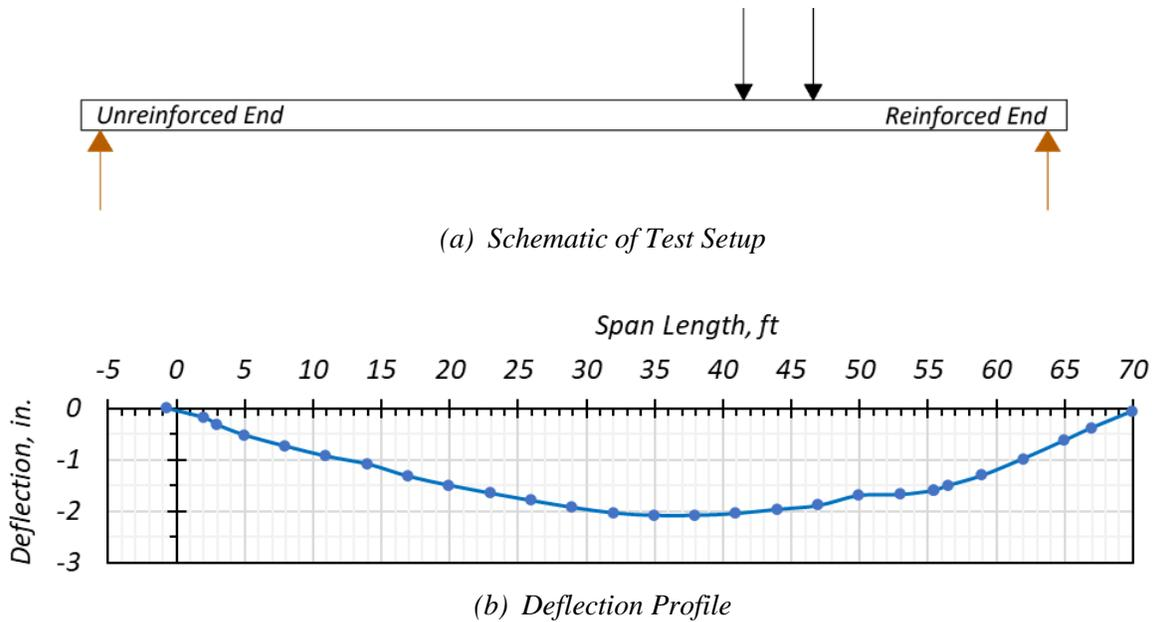
**Figure 6.53. Tx54 Shear Test 1: Deflection Profile.**
