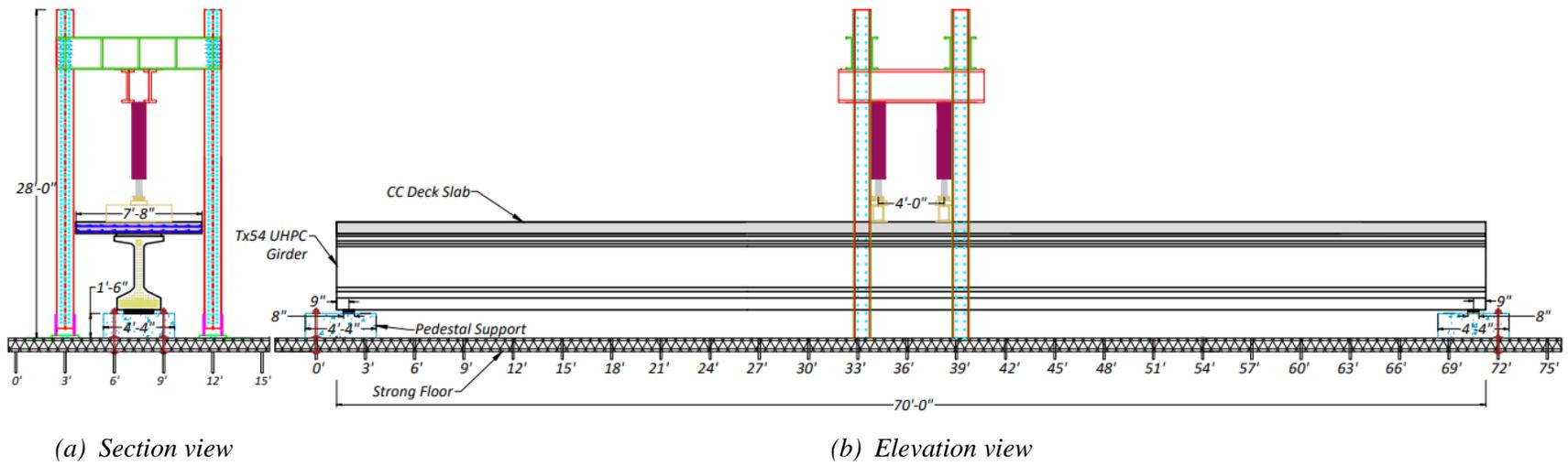
**Figure 5.4. Flexure Test Setup for Tx54 Girder.**
