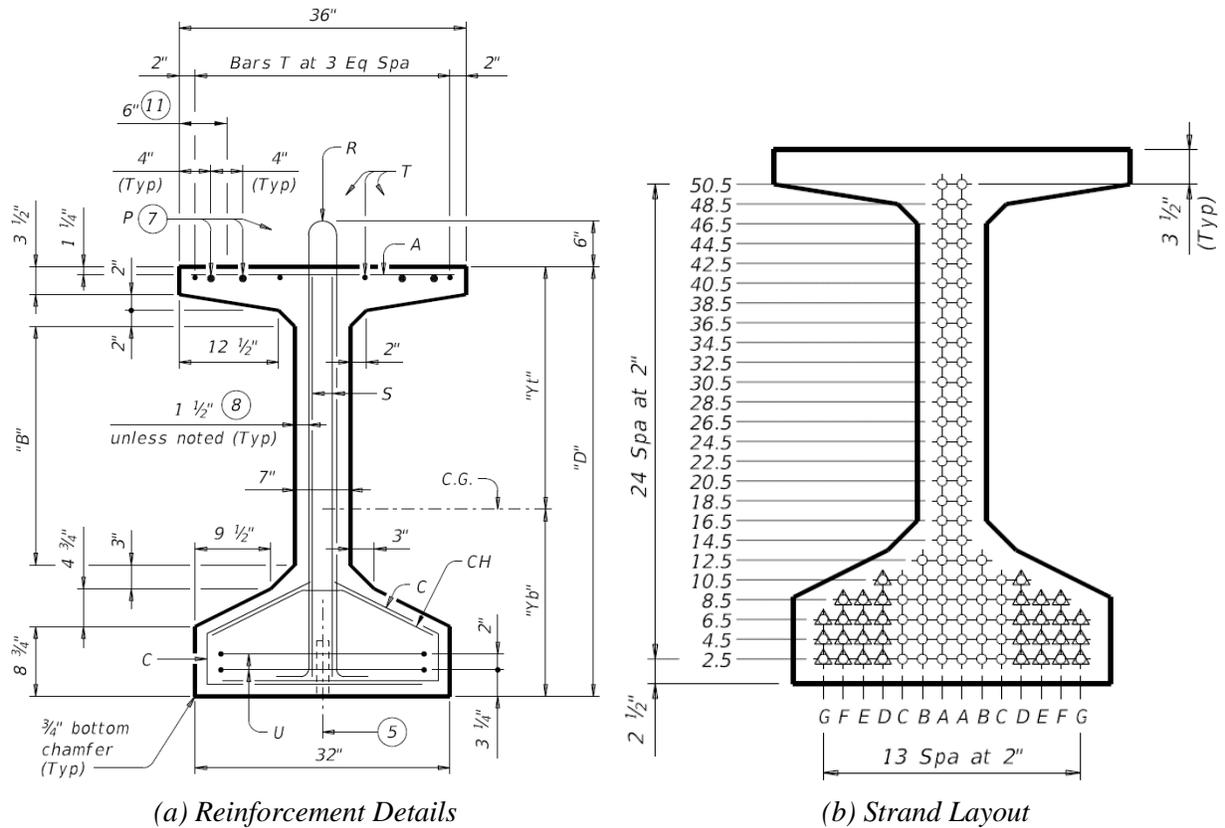
**Figure 3.16. Section Geometry of Tx54 Girder (TxDOT 2019).**
