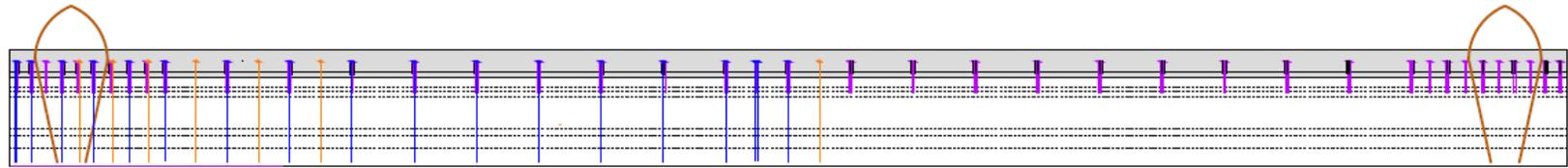
(a) Factored demand at 410 kips—No visible cracks
