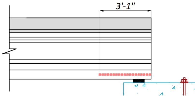
(b) Tx34-2 – 19 DEMEC Points at 2 in. Spacing
