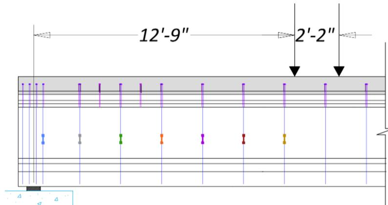
(a) Surface Steel Gages installed on R-bars
