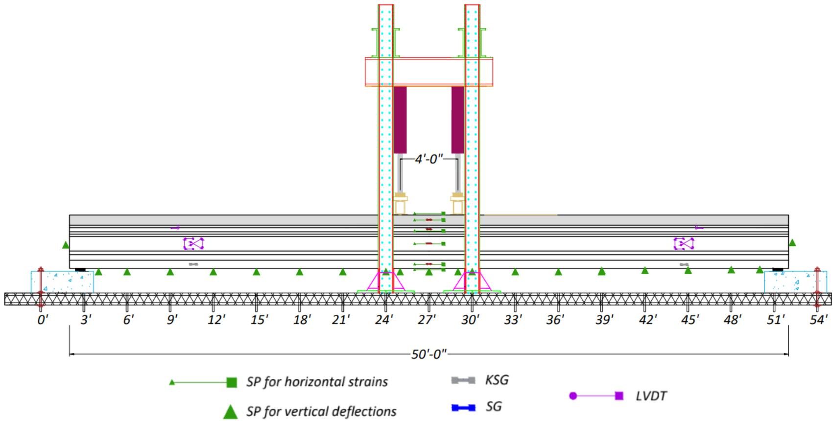
**Figure 5.6. Instrumentation for Flexure Test of Tx34-1.**
