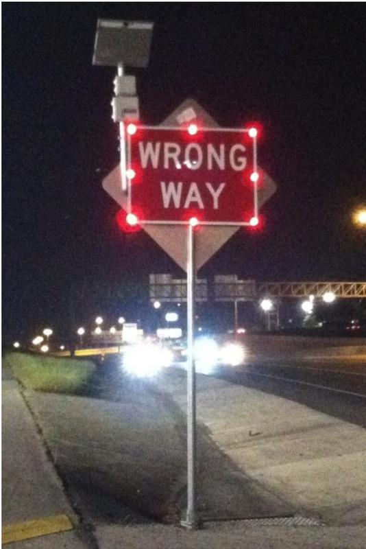
**Figure 1. WRONG WAY Sign with Red Flashing LEDs around the Border.**
