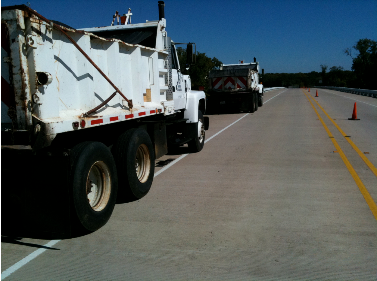
Figure 5.21. Load Trucks on Lane Stripe (Even Numbered Passes).
