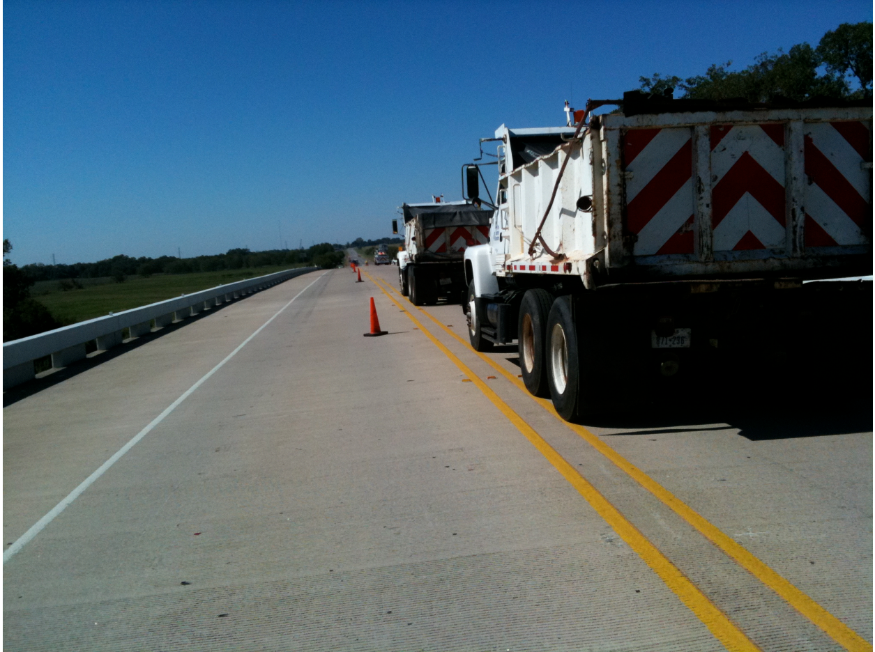
Figure 5.20. Load Trucks on Center Stripe (Odd Numbered Passes).
