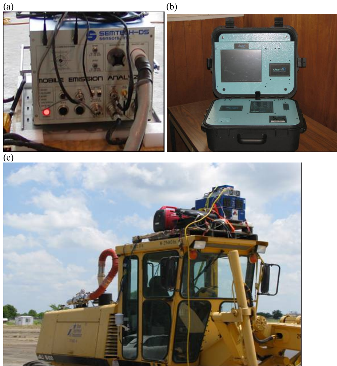
Figure 13. Emissions Measurement Instruments (a) SEMTECH-DS Unit, (b) Axion Unit, and (c) Both Units along with EFM Installed on a TxDOT Grader.
