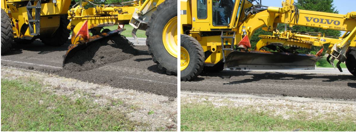
Figure 6. Grader Blade Position in forward (left) and backward (right) Movements.
