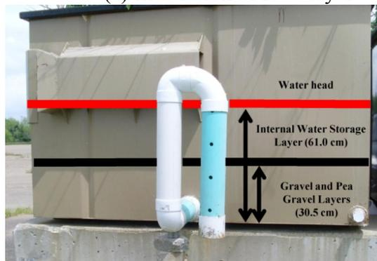
**Figure 3. Pilot Test Bioretention Boxes (Photos adapted from [Li et al., 2012](#)).**
