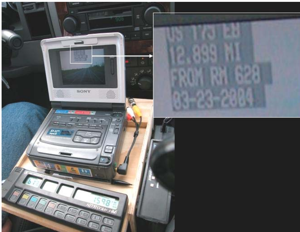
Figure 3-3. Example of DMI and Video Recording System along with Text Box of Information Recorded on the Video.
