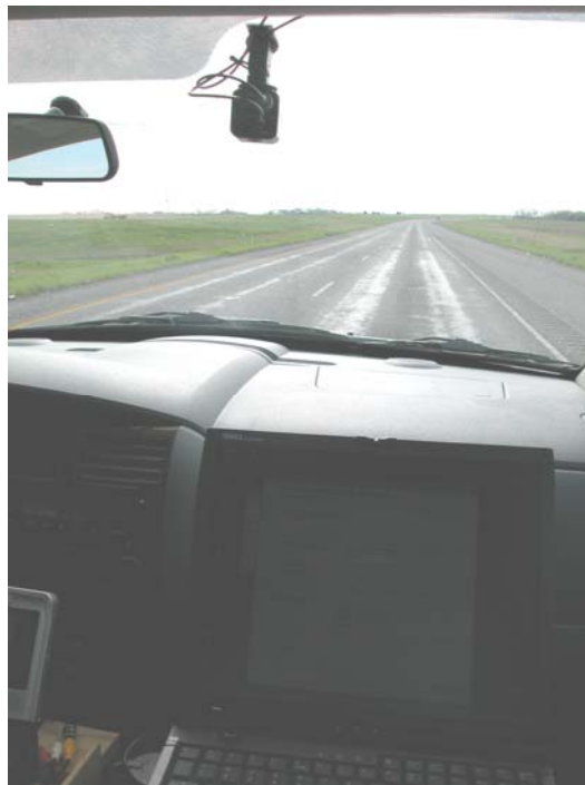
Figure 3-2. Example of Video Camera Mounted on Windshield.
