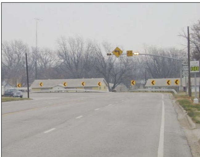
Figure 2. DSDS effect can be "lost" within other driver information sources at a site.
