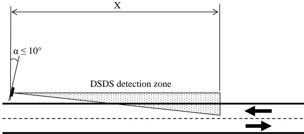
**Figure B-2. DSDS Installation Characteristics.**
