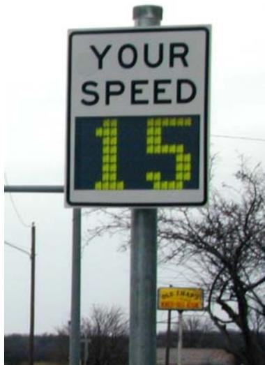
**Figure 2. Example of a Permanently Installed Self-Contained DSDS Unit.**
