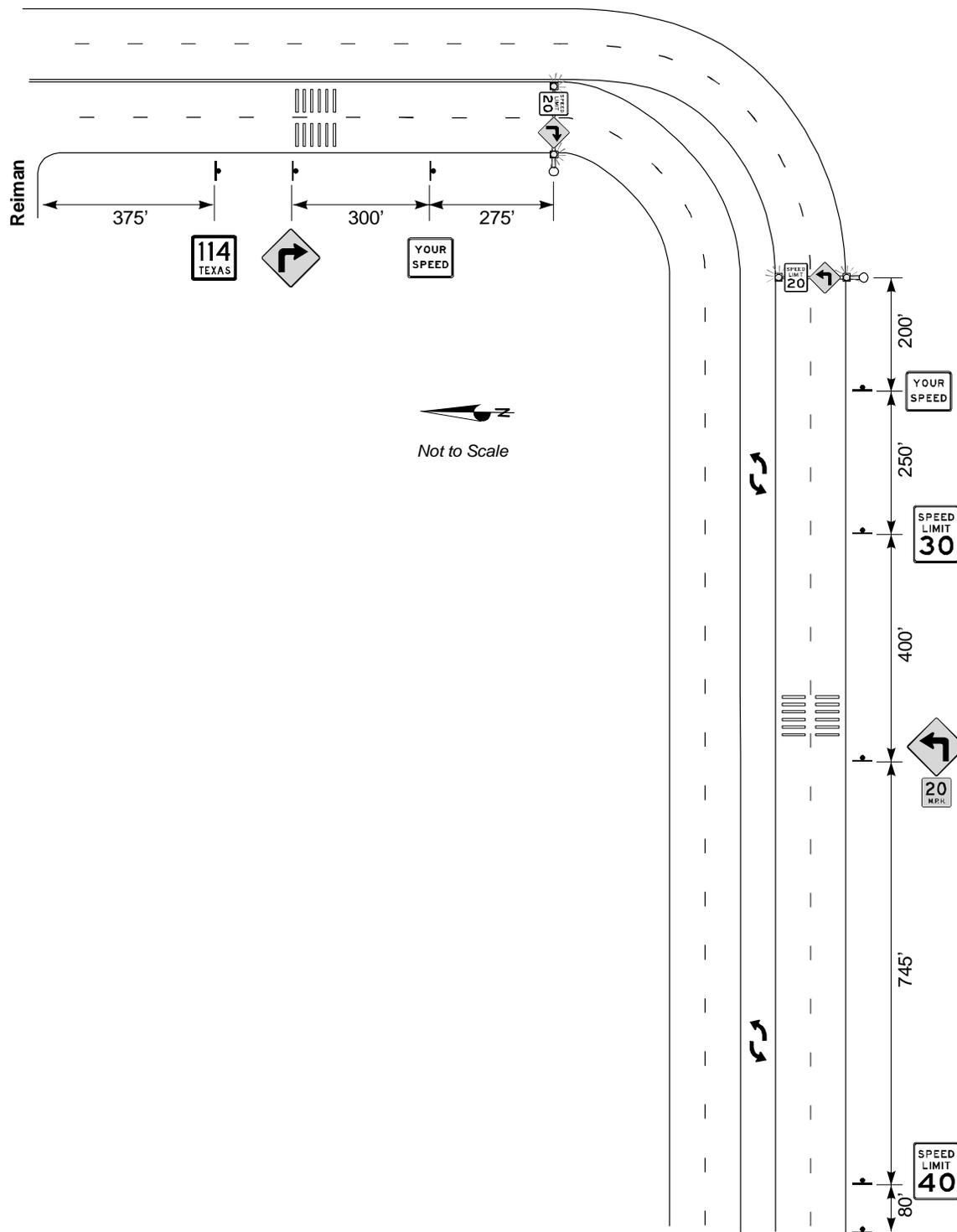
Figure 6. Schematic Layout of Sites 4 and 5.
