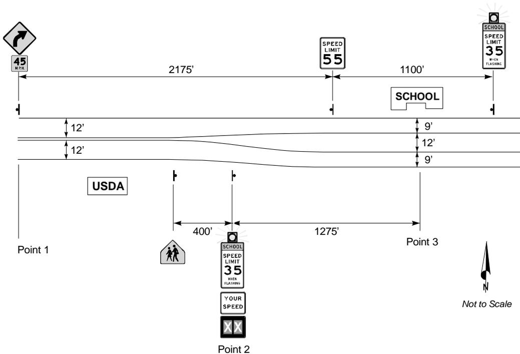
**Figure 3. Schematic Layout of Site 1.**
