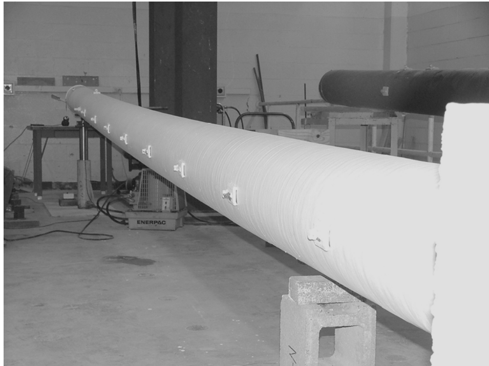
Figure 2.11 FRP pole deformed at 1 kips (4450 N)
