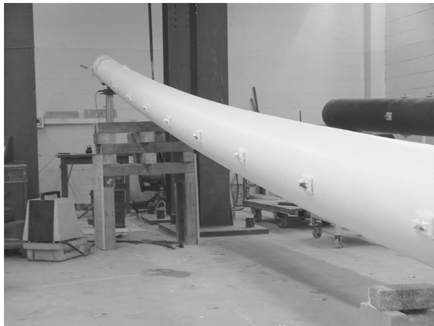
Figure 2.12 FRP pole deformed at 2 kips (8900 N)
