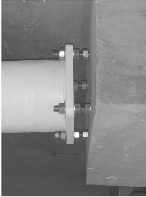
Figure 2.13 Bolt deformation at ultimate state
