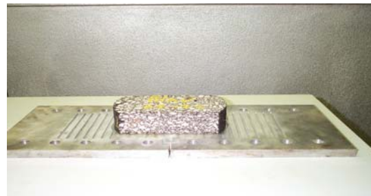
Figure 15. Test Specimen Glued to Plates.
