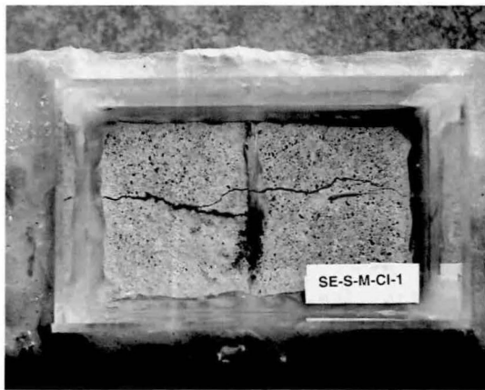
Figure 3.12 Top View of the Effect of a Faulty Epoxy Joint (SE-S-M-CI-1) Compared to a Sound Epoxy Joint (SE-S-L-CI-1)
