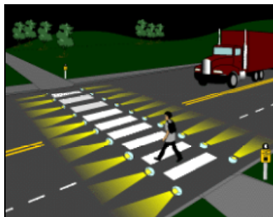
Figure 11. In-pavement Flashing Crosswalk Lights ( 20 )
