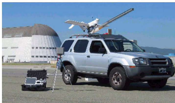
Figure 5. UAV Launch Device and Ground Station
