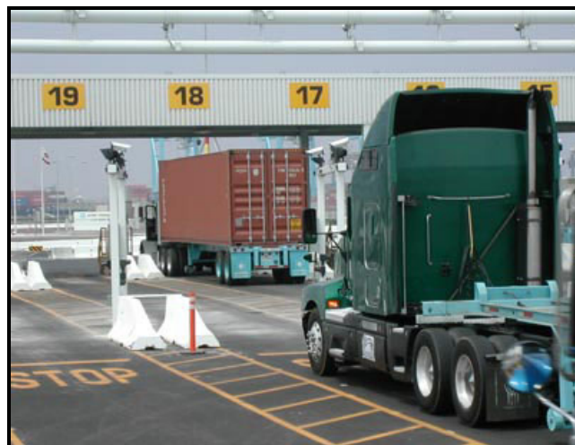
Figure 3. Rear View of Truck Entering Container Code Reader System ( 13 )
