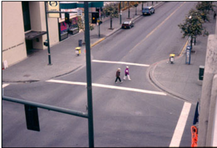
Figure 6. Curb Extension at an Intersection (Adapted from 16 )
