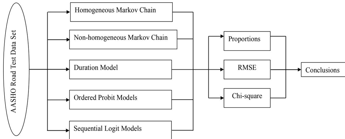
**Figure 6.1 Flowchart for Conducting the Comparison**
