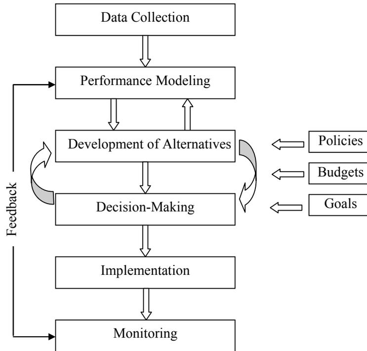
**Figure 2.2 Generic Pavement Management Process (CSI, 2002)**
