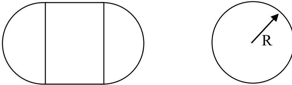
**Figure 5.5 Dimension of Tire Contact Area (Huang, 1993)**
