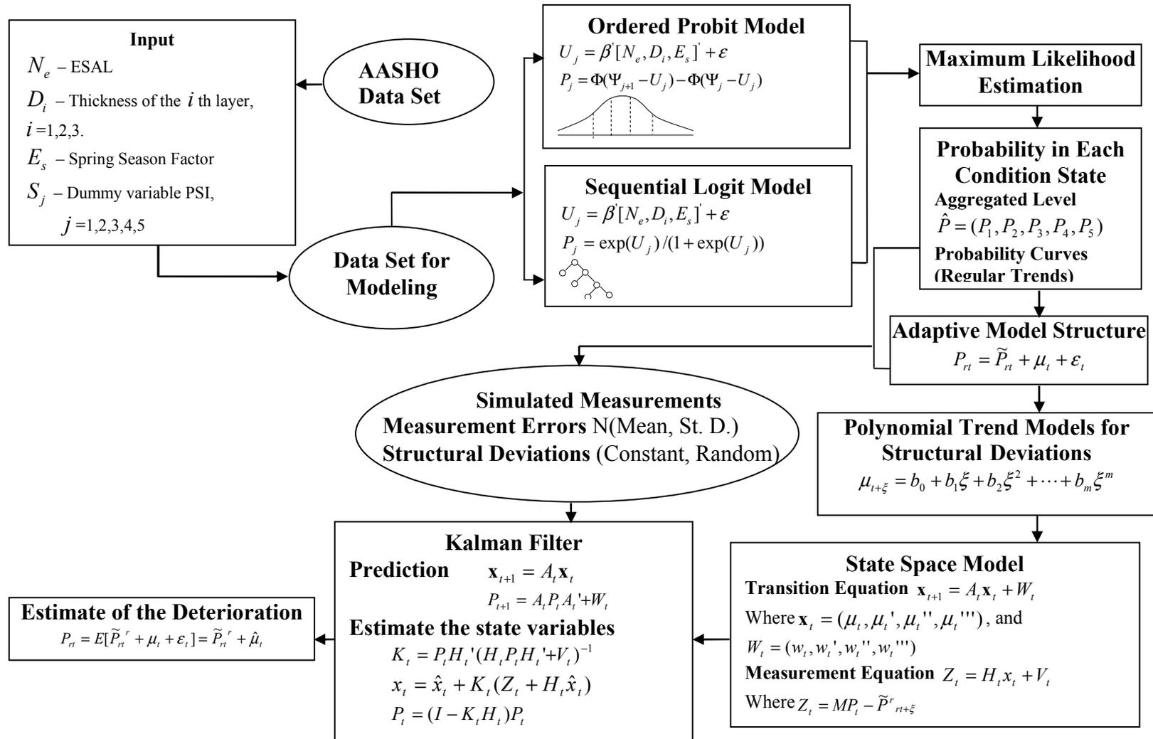
Figure 3.6 Major Components of the Methodological Framework
