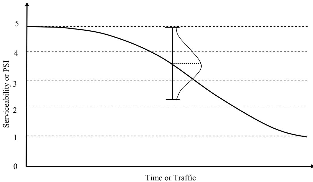
**Figure 3.2 Illustrations of Deterministic Models and Probabilistic Models**
