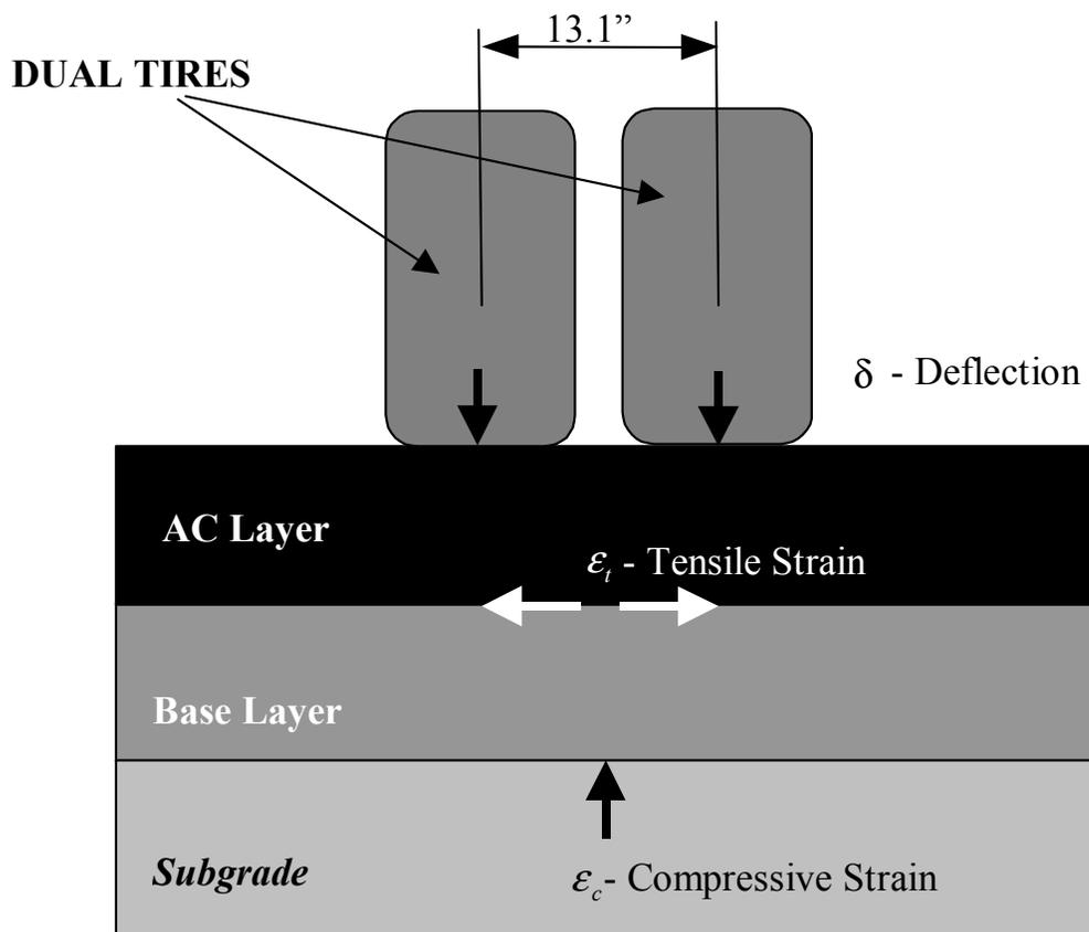
**Figure 5.4 Critical Primary Responses in Flexible Pavement Structure**
