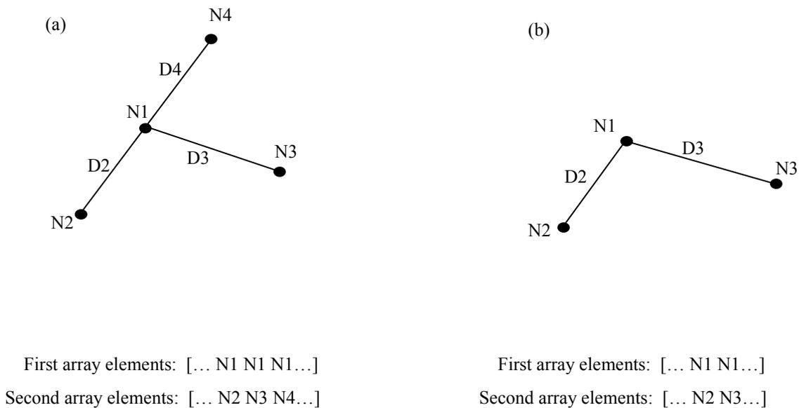
**FIGURE 21: Array representation for creating the sparse matrix**
