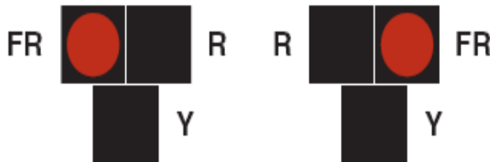
5. Alternating Flashing Red During Pedestrian Clearance Interval
